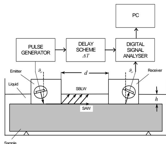
Fig. 1. The scheme of experimental investigations
