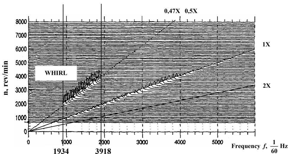
Fig. 7. Resonant frequencies of a rotary system with segmental sliding bearings, when clearance between the rotor and the bearing is 50  $\mu\text{m}$
