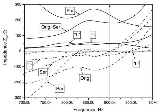
Fig. 11. Impedance changes after compensations
