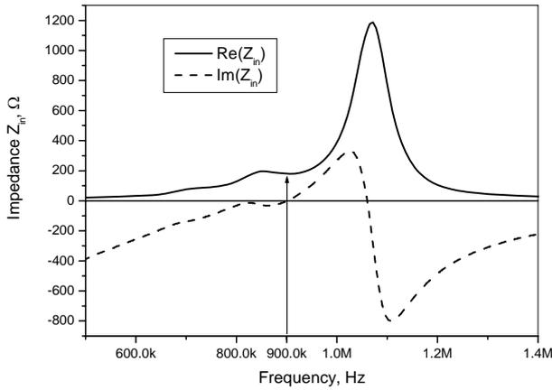
Fig. 7. Impedance after series inductance compensation
