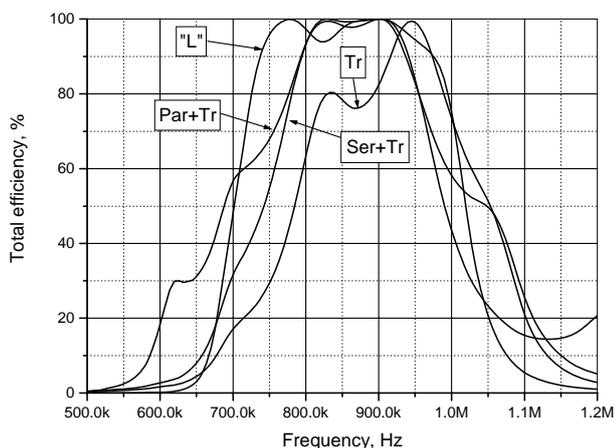
Fig. 18. Total efficiency for combined matching techniques
