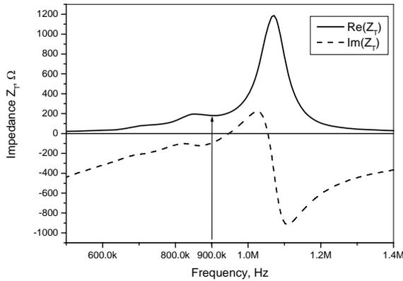
Fig. 4. Measured electrical impedance of ultrasonic transducer
