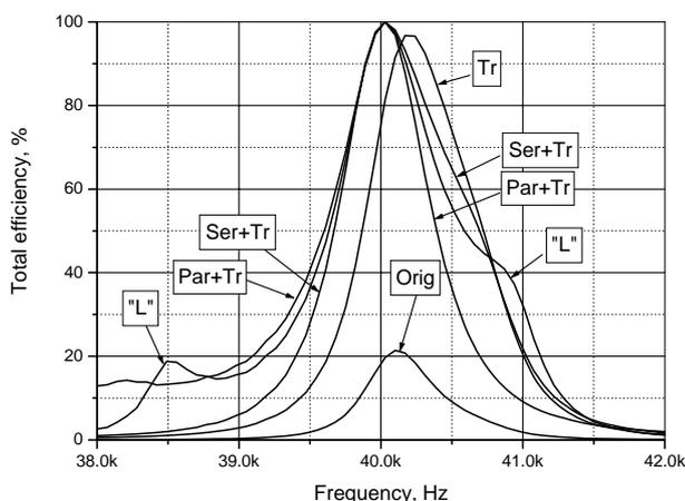
Fig. 19. Total efficiency for 40kHz commercial transducer.
