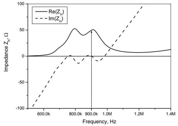
Fig. 9. Impedance after “L” matching
