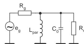
Fig. 2. Equivalent circuit with parallel compensating inductance
