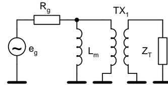
Fig. 10. Idealized transformer matching circuit
