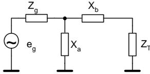
Fig. 8. Impedance after “L” matching
