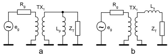
Fig. 17. Transformer matching combined with parallel (a) or series (b) inductance
