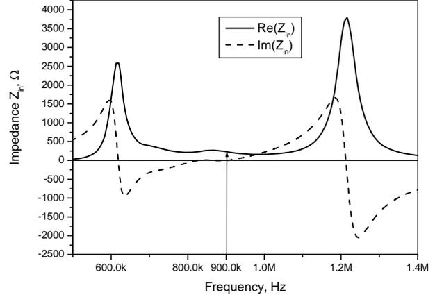
Fig. 5. Impedance after parallel inductance compensation
