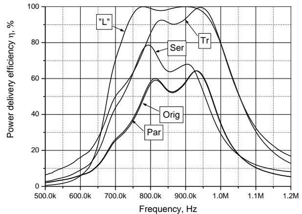
Fig. 13. Power delivery to load efficiency
