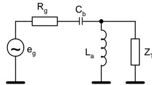
Fig. 16. “L” matching circuit for particular transducer
