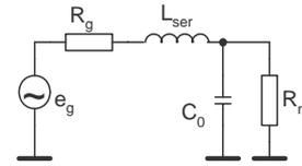
Fig. 6. Equivalent circuit with series compensating inductance
