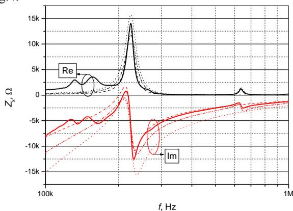
Fig. 4. Measured impedance approximation using the BVD model
