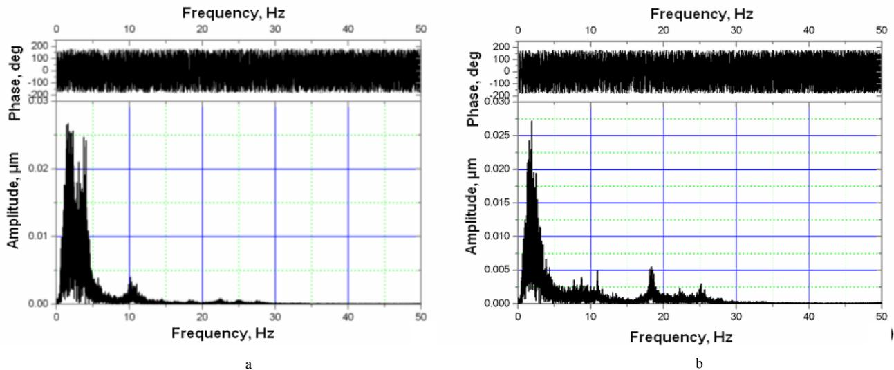
Fig. 4. The spectrum of the displacement signal at the point 4: a - horizontal direction, b - vertical direction.
