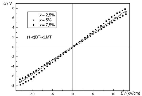
Fig.7. Dependencies of electric signal detected by BT-LMT plates with different composition on DC bias electric field
