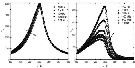
Fig.3. The temperature dependence of the real (a) and imaginary (b) parts of dielectric permittivity at different frequencies of BT-0.05LMT
