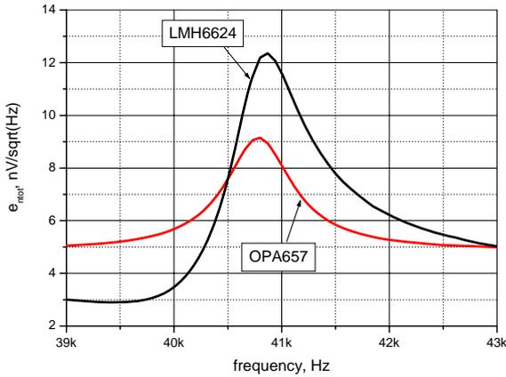
Fig. 4. Measured Prowave 400EP18D transducer voltage noise density
