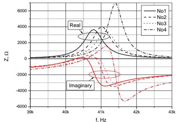
Fig. 3. Measured complex impedance of the Prowave 400EP18D transducer
