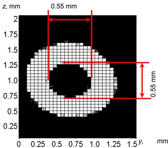
Fig. 10. The image of the reflection from the metallic ball, formed by acoustic lenses system. The ball's position is 2 (Fig. 7)
