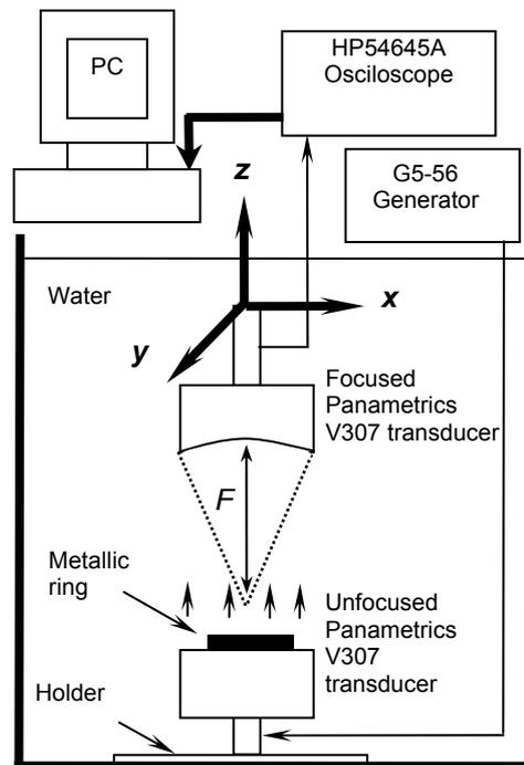
Fig. 13. The experimental set-up for the scanning of the ultrasonic field, emitted by the plane transmitter with placed on metallic ring measurements of the planar transducer ( $F$  – focus length of the focused transducer)
