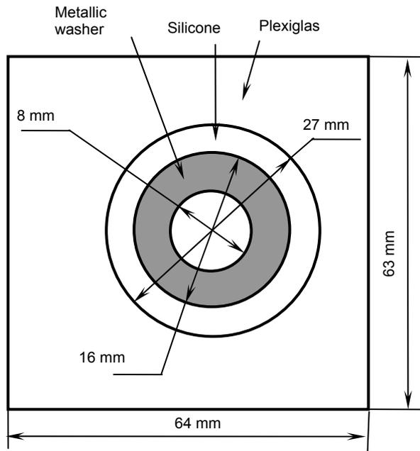
Fig. 1. The test sample with a washer, embedded in silicone, provided by the manufacturer. The thickness of the test sample is 9 mm
