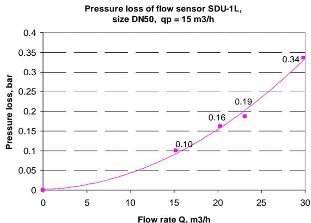
Fig. 3. The pressure loss of the flow sensors SDU-1L, size DN50 with flow conditioning swirl pins. Pressure loss at permanent flow rate  $q_p=1.5$  m<sup>3</sup>/h is 100 mbar (maximum permissible pressure loss at permanent flow rate is 250 mbar). Pressure loss has been measured with differential pressure transmitter Fuji Electric FCX-CII.
