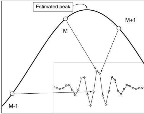
Fig. 2. The parabolic interpolation for TOF estimation
