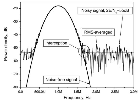
Fig. 3. The power spectral density of the simulated signal
