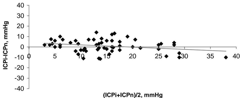
Fig. 7. Bland - Altman plot (57 simultaneous invasive and non-invasive aICP measurements in ICU): mean value  $m = ICP_i - ICP_n = 0.939$  mmHg, standard deviation  $SD = 6.18$  mmHg, solid line shows a negligible systematic error of the non-invasive aICP measurement system.
