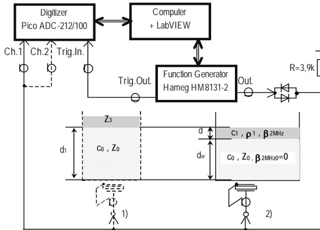
Fig. 1 The structure of experimental system setup
