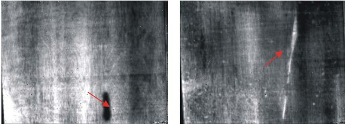
**Fig. 7:** Two thermographic images during the process of décor paper laminating of plywood. The left image shows a fallen off branch in the center layer of a 5 mm thick plywood and the right image shows a faulty gluing at the veneer joints of the last layer of the plywood.
