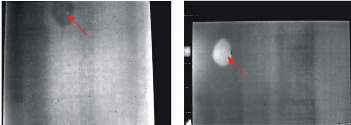
**Fig. 6:** Two thermographic images with splitting in the particleboards. One splitting in the lower surface layer of the 22 mm thick particleboard shows as a dark (cold) spot (left image) and another splitting in the upper layer of the board shows up as a white (hot) spot (right image).
