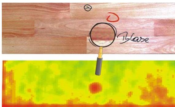
**Fig. 4:** Photo of a laminated flooring with no visible defect on the surface (top) and thermographic image (bottom) with a blister shown as red (hot) spot and poor adhesive bonding shown as irregular red areas.
