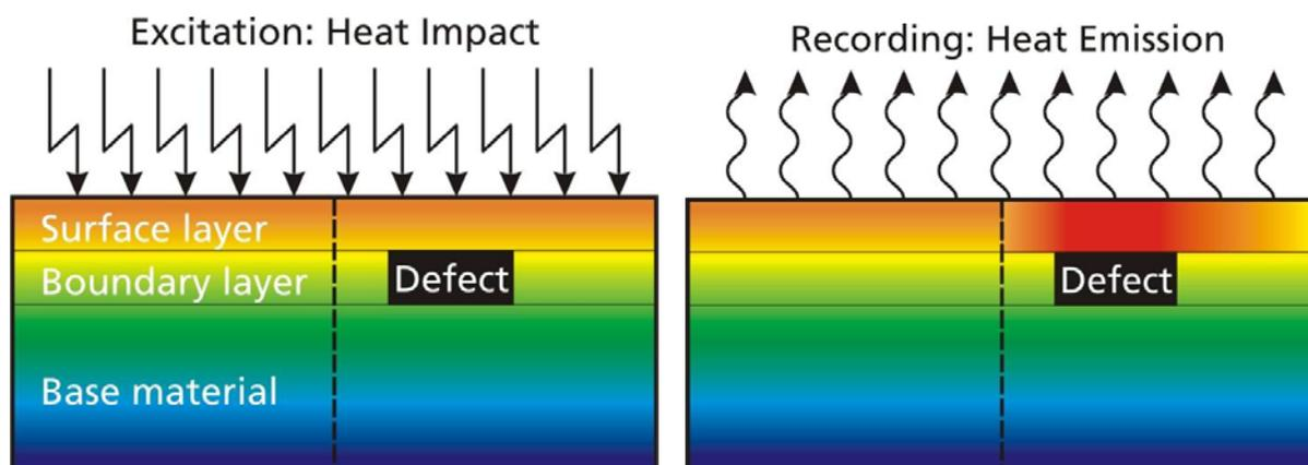
**Fig. 1:** Schematic drawing of the principle of infrared thermography, showing the uniformly distributed heat impact on the surface (left), the recorded heat emission (right) and the warmer region (dark) on the surface above the defect.
