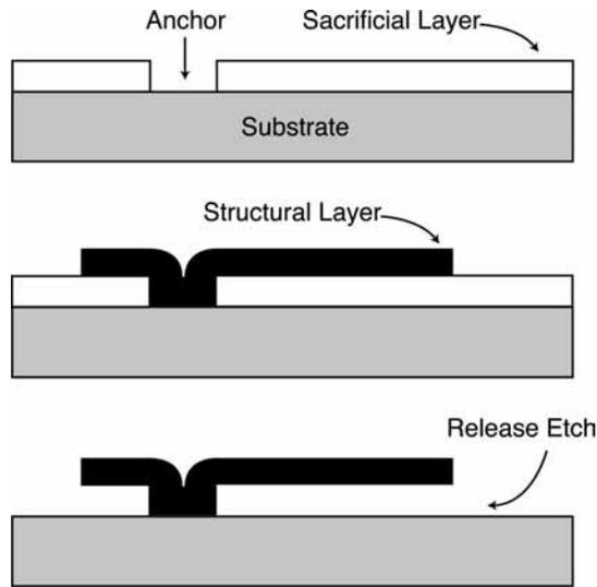
**FIGURE 3 Surface micromachining**
