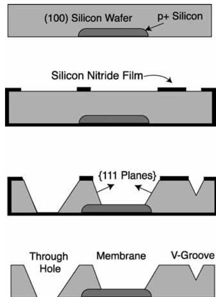
**FIGURE 4 Bulk micromachining**
