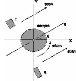
Fig. 1. The conventional CT scanning technique.
