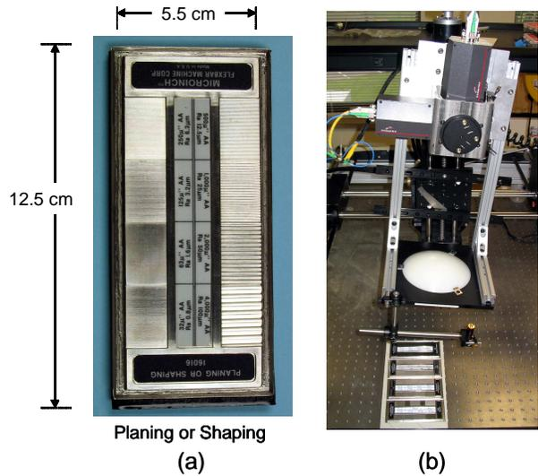
**Figure 5.** One of the comparator plate used in the surface roughness measurements (a) and the confocal head shown tilted at a 5 degree angle from normal.
