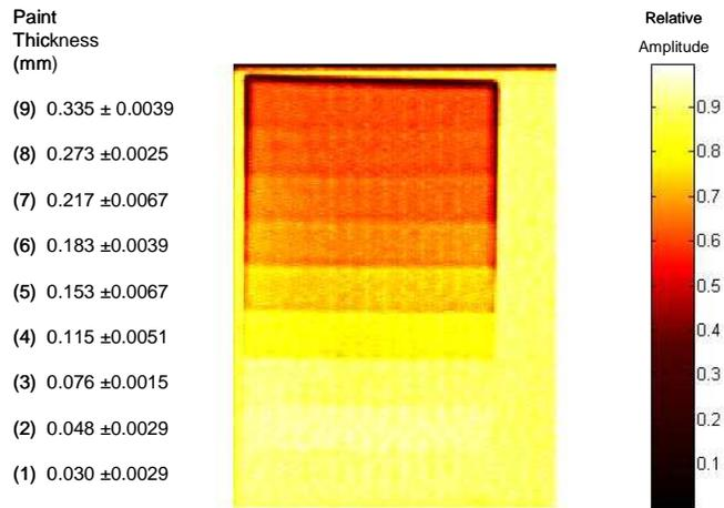
**Figure 4.** THz Amplitude Image (maximum signal amplitude).
