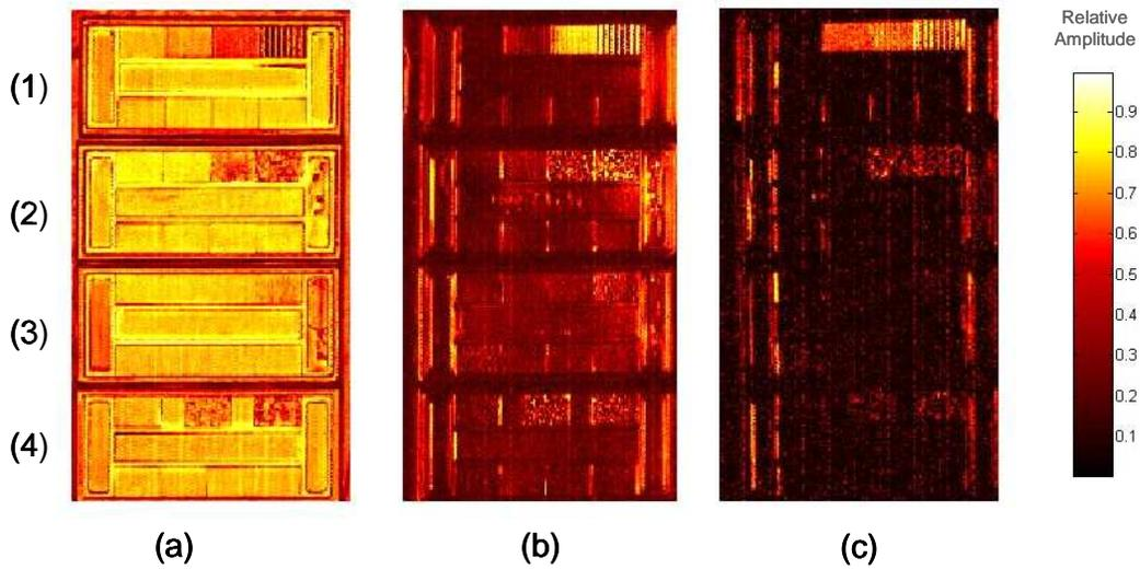
**Figure 6.** Comparator plate frequency images for the THz head at (a) 0 deg, (b) 10 deg, (c) 20 deg. Plate-1 is the Planning and Shaping, Plate-2 is EDM, Plate-3 is Grit and Shot Blasting, and Plate-4 is Casting.
