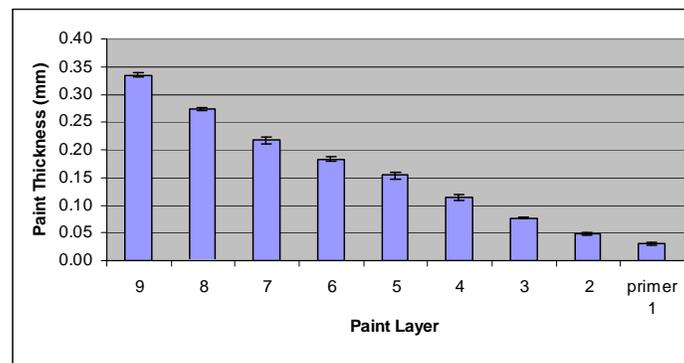
**Figure 2.** Paint layer thicknesses on an aluminum substrate.
