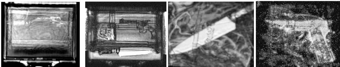
**Fig. 3** Reflection terahertz images. From Left: Return from top of case attaché case; return from interior of case showing knife and pistol; knife under jacket; pistol under jacket.
