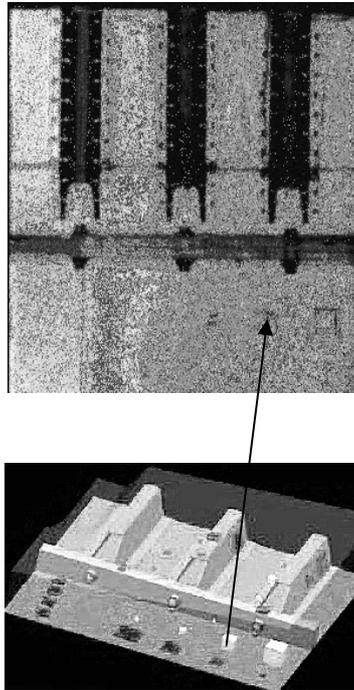
**Fig. 5** Terahertz images of space shuttle external tank mock-up panel with programmed synthetic voids and disbands. Top: High resolution image of synthetic voids and disbands. Bottom: 3D view of programmed location of voids on panel. The 3 structures at top are known as “stringers”, the structure from left to right with the 3 bolts is the “flange”
