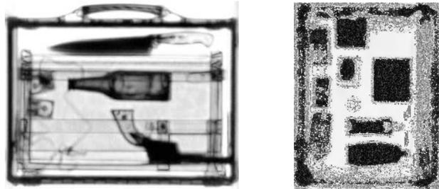
**Fig. 2** Transmission terahertz images. Left: Attaché Case. Right: Suitcase, approx. 30 in. by 20 in, by 13 in.
