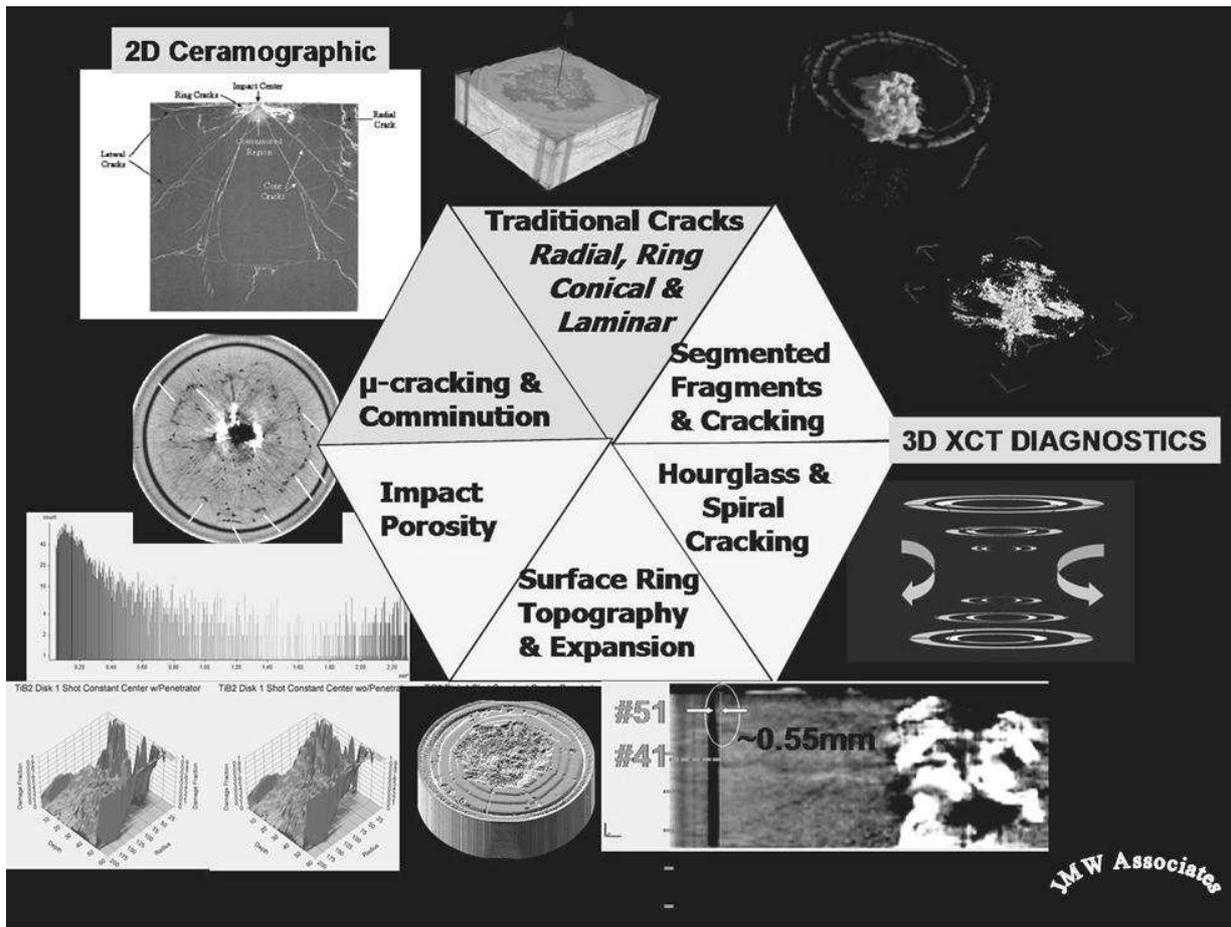
Figure 1. Representative examples of terminal ballistic impact damage details including those observed with both traditional destructive sectioning and those more fully characterized with non-invasive XCT damage diagnostic techniques.
