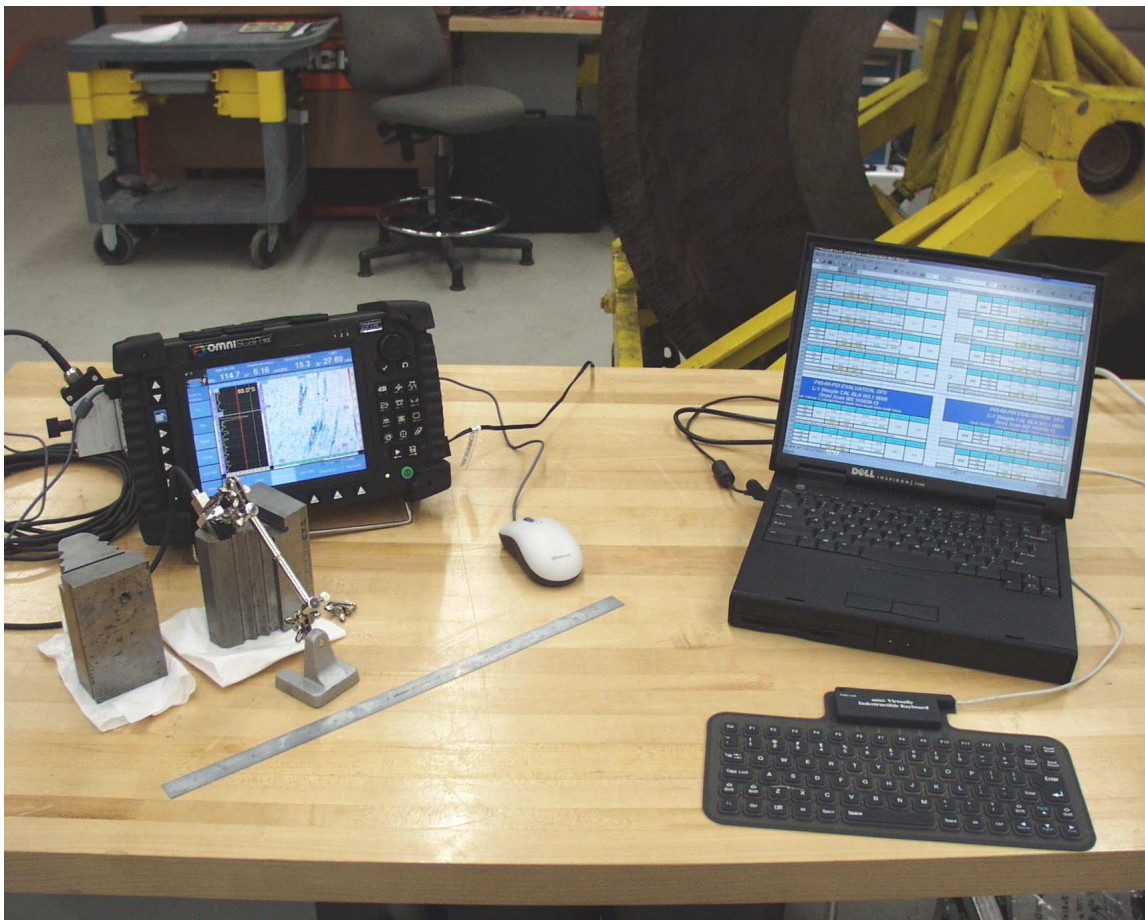
Figure 1: Example of experimental set-up for probe 43+60T on L-1 steple PDI coupons.
