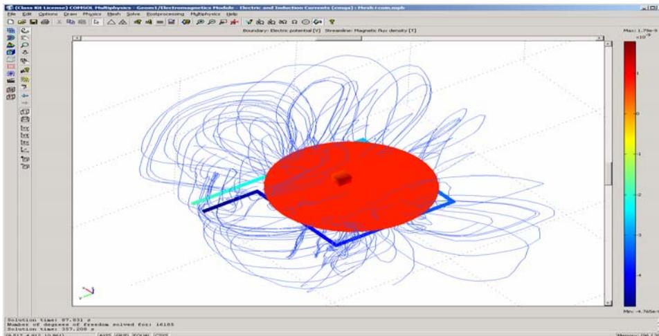
**Figure 11:** Magnetic flux lines for Mesh sensor obtained from FE model Medium Conductivity
