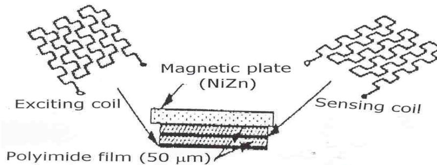
**Figure 2:** Structure of the Mesh type sensor
