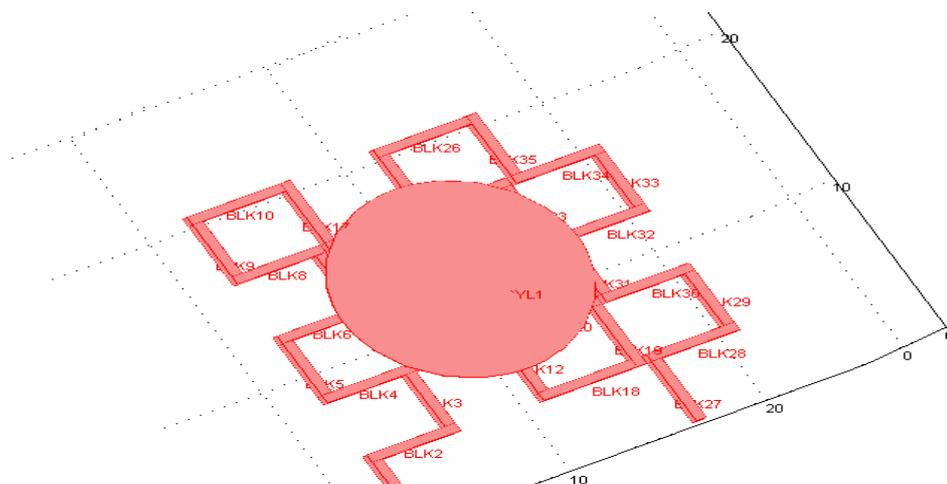
**Figure 9:** Finite Element Model for coin testing for mesh type sensor
