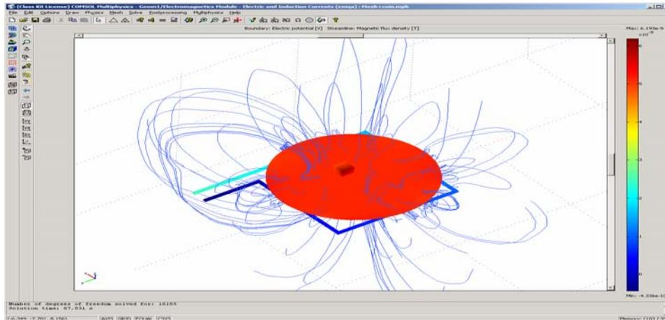
**Figure 10:** Magnetic flux lines for Mesh sensor obtained from FE model (Low Conductivity)
