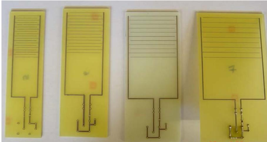
**Figure 6:** Fabricated interdigital type sensors, four sizes
