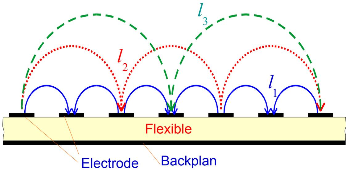
**Figure 3:** Field distribution of planar interdigital type sensor
