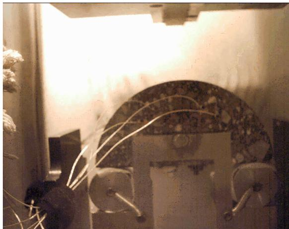
Figure 6. Asphalt specimen in the testing chamber.
