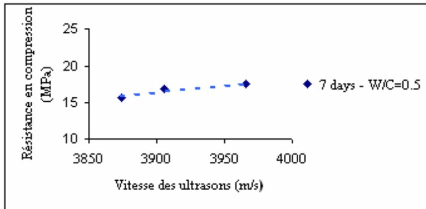
Fig. 5 Relations between ultrasonic velocity and strength at 7 days (W/C=0.5)
