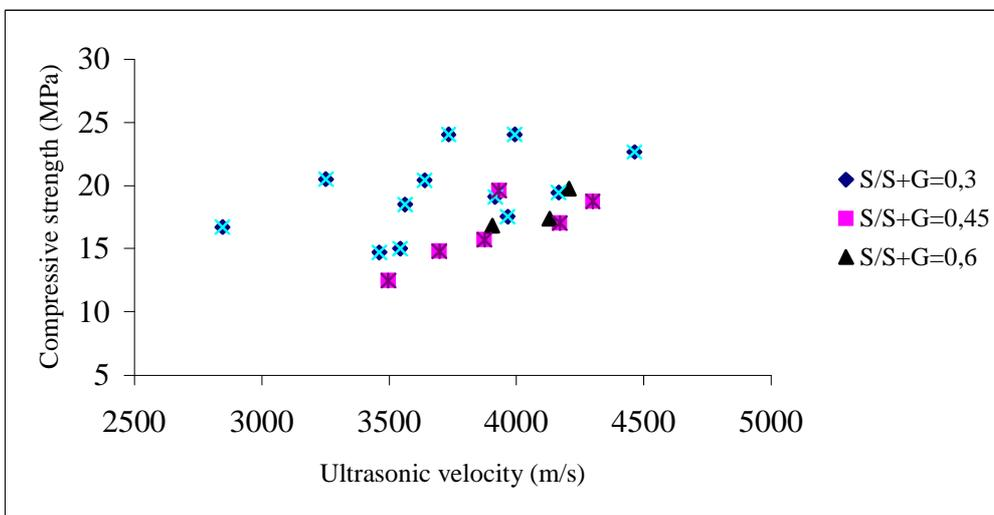
Fig. 4 Relations between ultrasonic velocity and compressive strength for various ratios S/S+G
