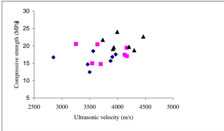
Fig. 1 Relations between ultrasonic velocity and compressive strength at the various ages
