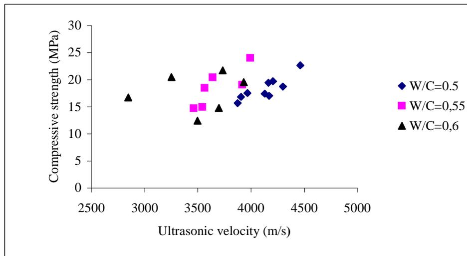
Fig. 3 Relations between ultrasonic velocity and compressive strength for various ratios E/C
