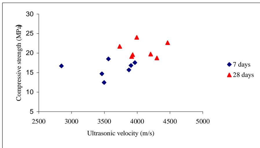
Fig. 2 Relations between ultrasonic velocity and compressive strength at 7 and 28 days
