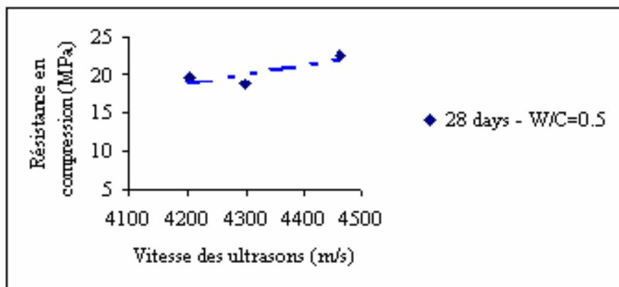
Fig. 6 Relations between ultrasonic velocity and strength at 28 days (W/C=0.5)
