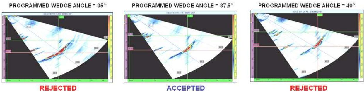
**Figure 11:** Example of crack detection and sizing by three set-ups with programmed wedge angle: 35° (left), 37.5° (actual-middle), and 40° (right).
