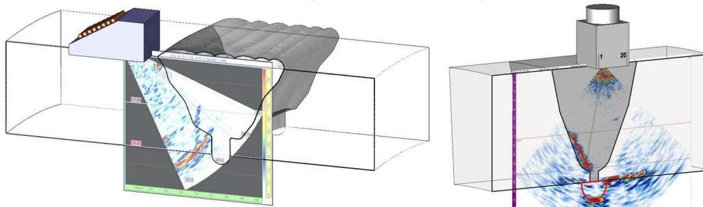
**Figure 11:** Example of 3-D data plotting of a toe crack (*left*) and of an embedded crack (*right*).
