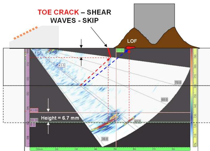
**Figure 9:** Example of toe crack and LOF detection and plotting using the skip. Omniscan data crack height is 6.7 mm vs. 6.8 mm actual height.
