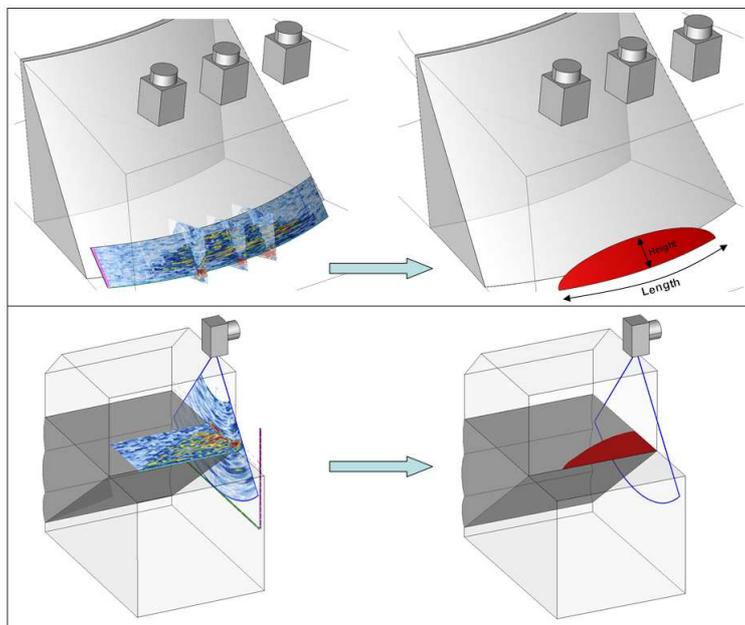
**Figure 14:** Example of defect reconstruction based on B- and S-data.
