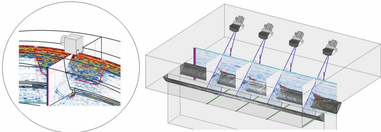
**Figure 15:** Example of data plotting of B-and S-scan into a piping weld for a crack detected with L-waves (*left*) and for four implanted toe cracks detected with shear waves (*right*).
