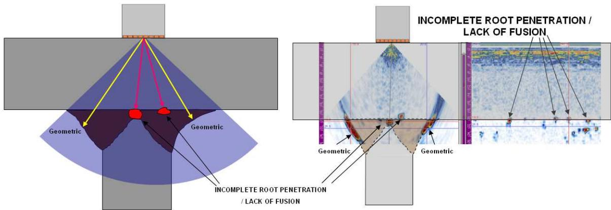
**Figure 6:** Data plotting for a T-weld S-scan display representing incomplete root penetration and lack of fusion detected by a direct-contact longitudinal waves probe.
