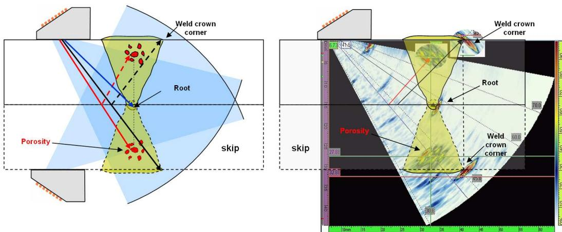
**Figure 5:** Principle of detection (*left*) and 2-D data plotting of Omniscan S-scan in detecting a nest of porosity with skip.
