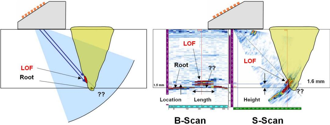
**Figure 2:** 2-D data plotting for a LOF located near the inner surface. A combination of B-and S-views provide the LOF parameters (location, length, height, orientation). *Left:* detection principle and shadowing effect of the root signal; *right:* 2-D data plotting for S-scan; B-scan was added for length and inner ligament measurements.
