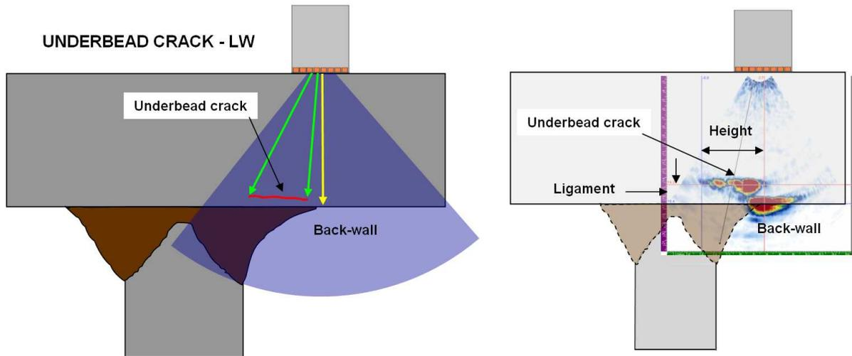
**Figure 7:** Principle of detection (*left*) and S-scan data plotting for an underbead crack located in a T-weld.
