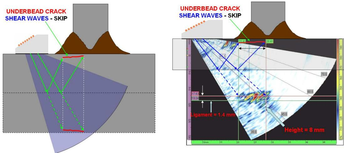
**Figure 8:** Example of S-scan data plotting for Omniscan –shear waves - in detecting the underbead crack from Figure OPG-7. *Left:* principle; *right:* data plotting.
