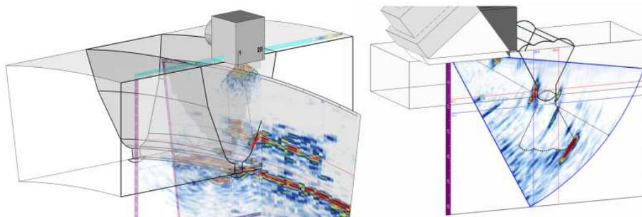
**Figure 12:** Example of data plotting for LOF using L-waves (*left*) and T-waves (*right*).
