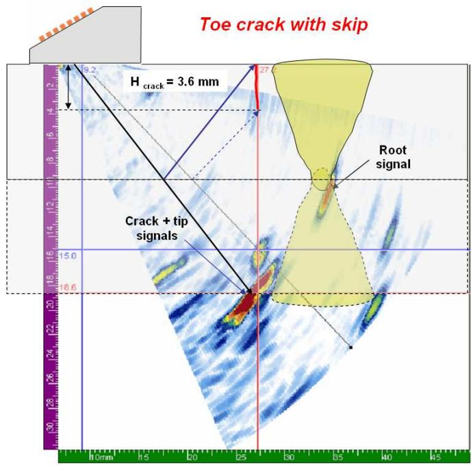
**Figure 1:** 2-D data plotting of a S-scan image in detecting and sizing a toe crack. Detection was performed with skip. The crack height is measured from corner trap to the last diffracted signal of crack tip. Actual crack height is 3.8 mm.
