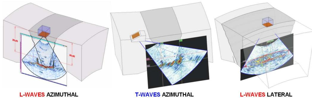
**Figure 10:** Examples of 3-D data plotting of S-scan display into isometric part.
