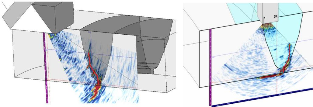
**Figure 13:** Example of data plotting for an inner-surface crack detected with shear-waves probe (*left*) and with an L-waves probe (*right*).
