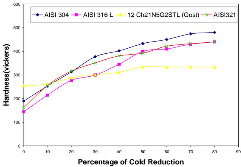
Fig 4:- Variation of hardness as a function of cold reductions.
