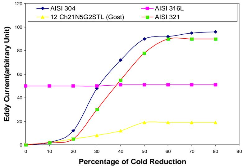
Fig 1-; Variation of eddy currents as a function of cold reductions.
