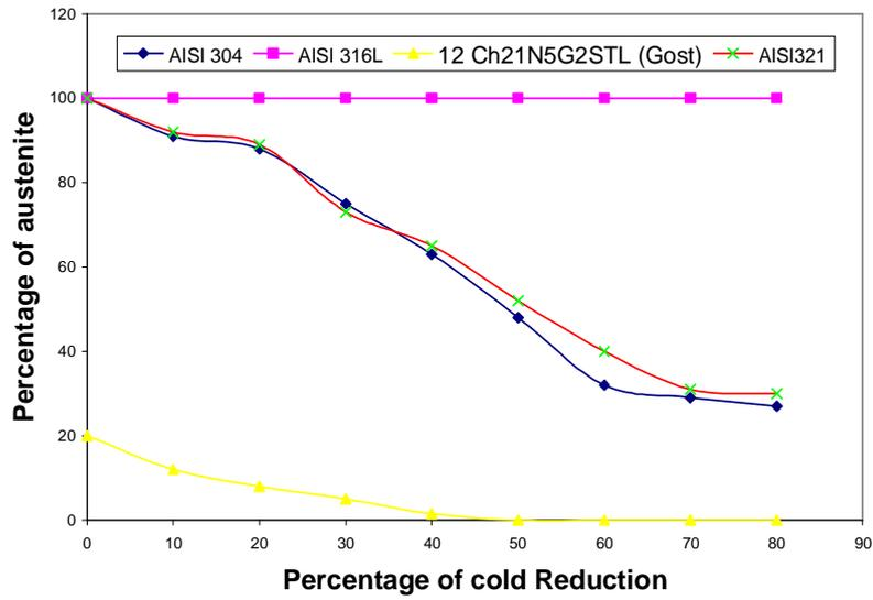
Fig 2-: Variation of austenite as a function of cold reductions.
