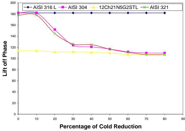
Fig 3:- Variation of lift off as a function of cold reductions.
