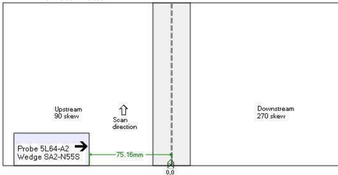
These graphic screen captures and parameters are extracts from a demonstration report generated by ESBeam Tool. The software gives the operator all the documentation tools necessary to generate a complete scan plan according to ASME and most UT inspection codes requirement.
