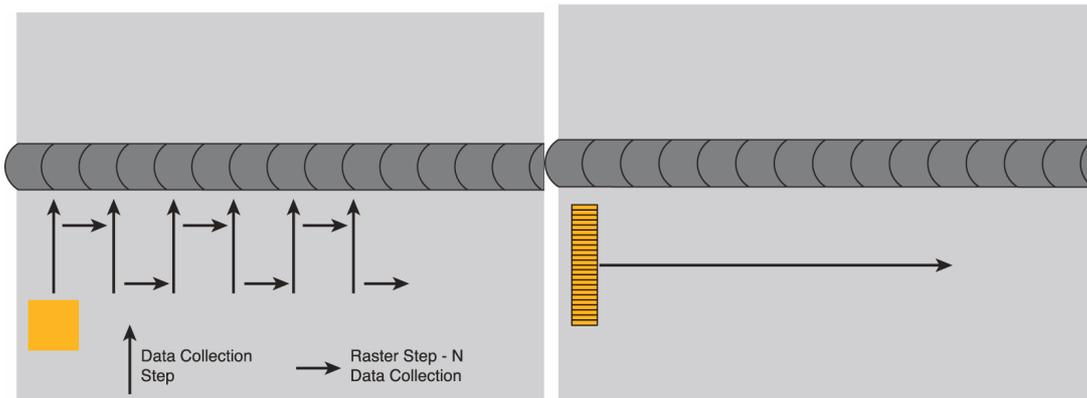
Figure 2a (left), conventional raster scanning. Figure 2b (right) linear scanning.
