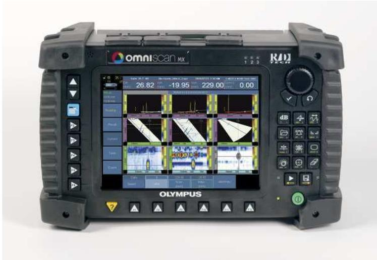
Figure 3: Multigroup screen display from OmniScan MX for encoded scanning. Note that other manufacturers also produce encoded portable phased array units.
