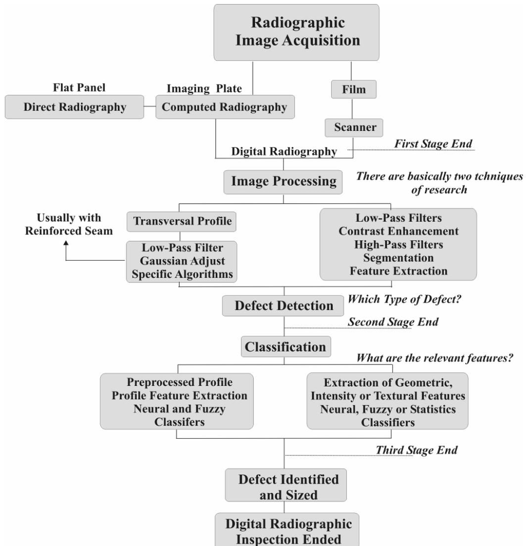
FIGURE 2: Stages of Automatic Inspection of Weld Seam by Digital Radiography.
