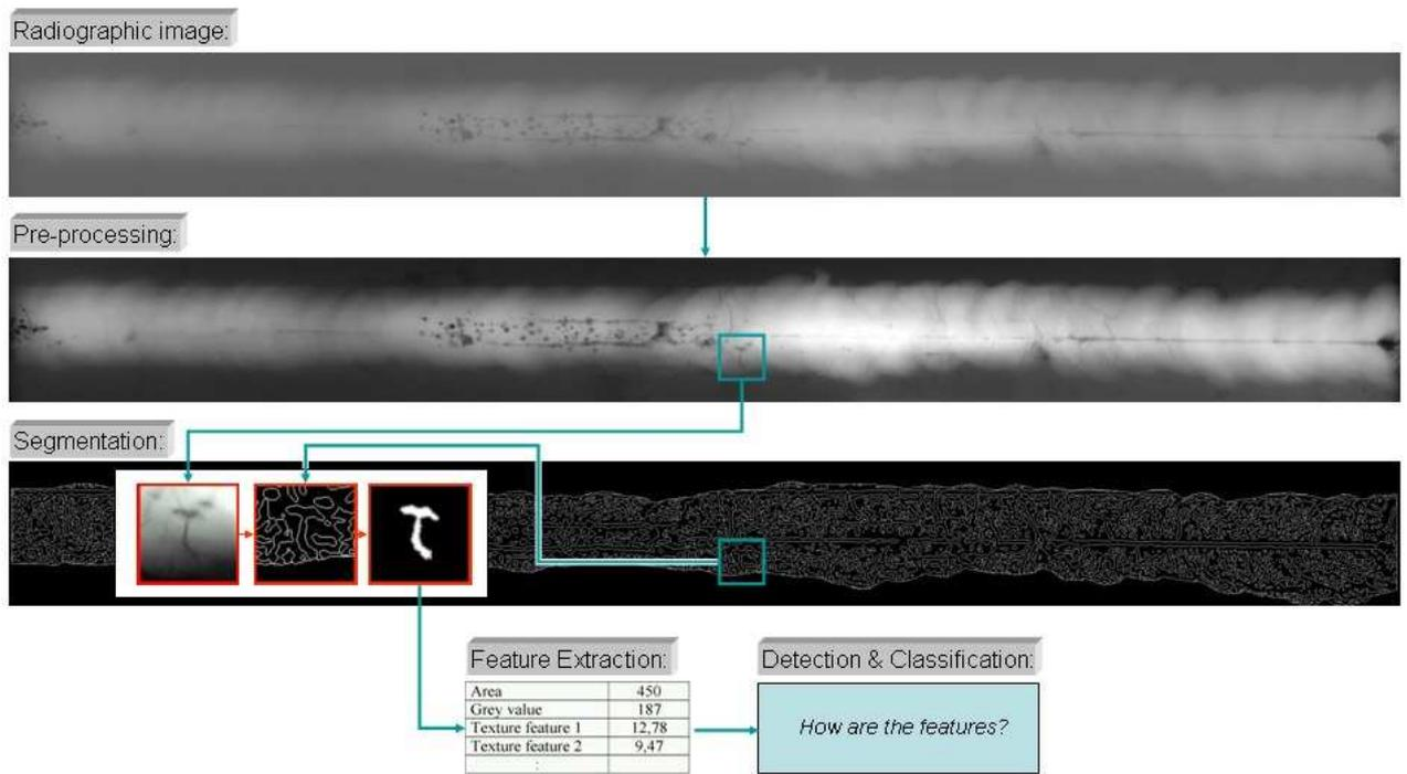
**FIGURE 1:** Schematic diagram of the detection of defects in welds.
