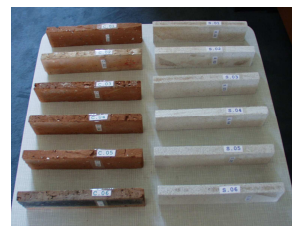
Picture 5 Specimens of ceramics ware and gas concrete conditioned to surveying [3]
