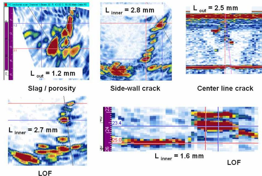
**Figure 7:** Examples of ligament measurement for different weld flaws.
