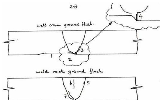
**Figure 2:** Example of implanted defects in mock-up TP 9 (  $\varnothing$ 365 mm x 24 mm).
