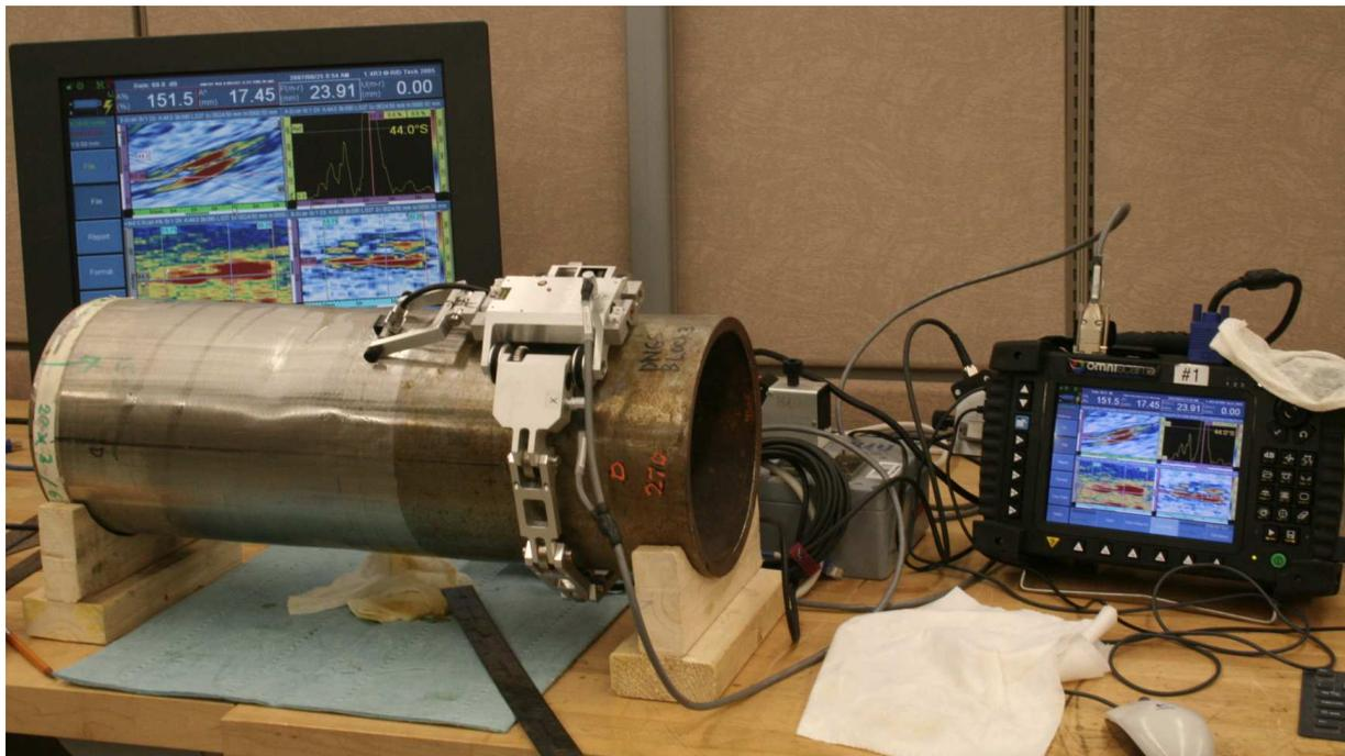
**Figure 3:** Example of experimental set-up for sizing capability on dissimilar piping weld mock-up DNGS BLOCK #3.
