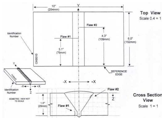
**Figure 1:** Example of implanted defects in a welded plate.
