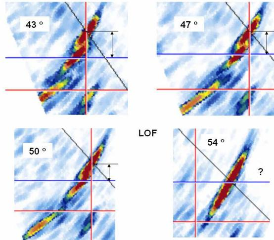
**Figure 6:** Example of the influence of detection angle on LOF sizing capability (one-side examination).
