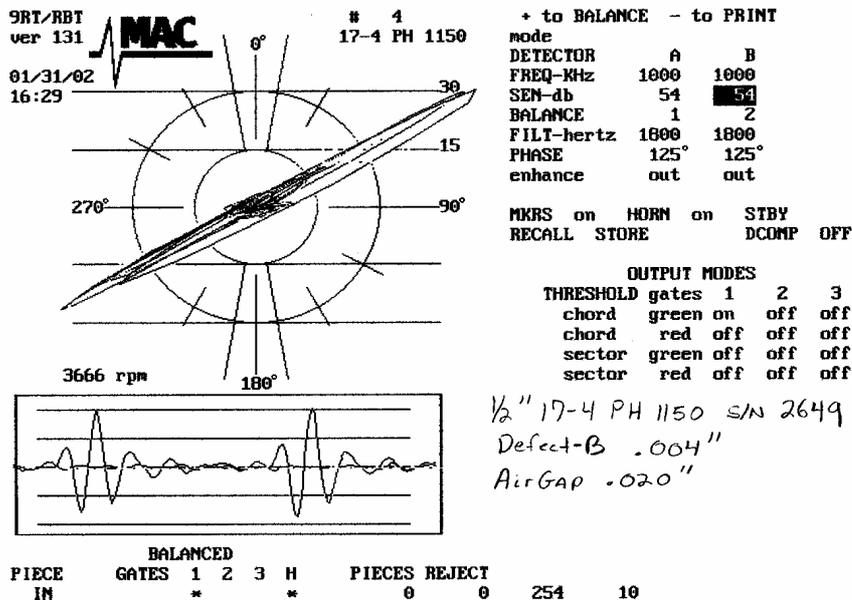
FIG 9 - .004" flaw in 17-4 PH Testing this same material at 1MHZ made a very difficult test simple. The noise signal is in the same plane as the flaw signal response at this frequency.
