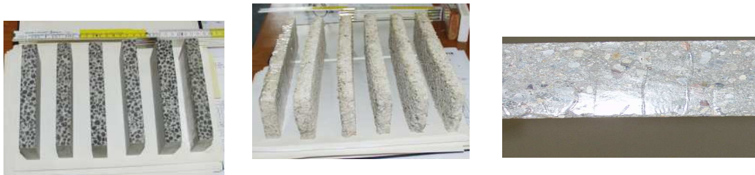
Pic. 1 Material samples developed at TSHD FAST VUT Brno – “R” concrete (left), “H” material (middle), “R 0” concrete (right) [4]
