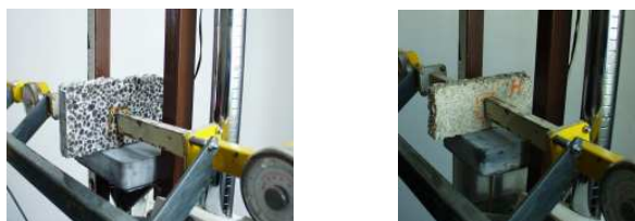
Pic. 06 "R" concrete and "H" material during measurement to assess function dependency for EMW radiation (mV) intensity change according to the specific moisture.
