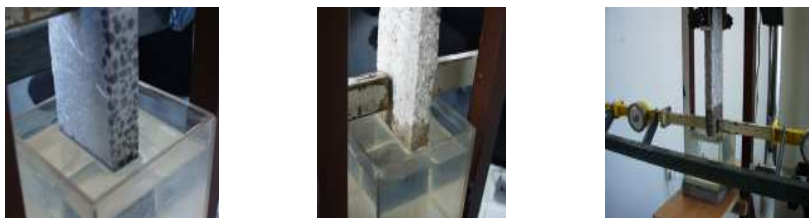
Pic. 2 Position of the “R” concrete, “H” materials and “R 0” concrete samples during moisture behavior monitoring
