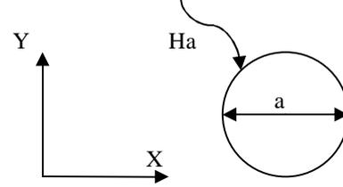
Figure 3. System of coordinates for the calculation of the magnetic flux leakage of a subsurface flaw.
