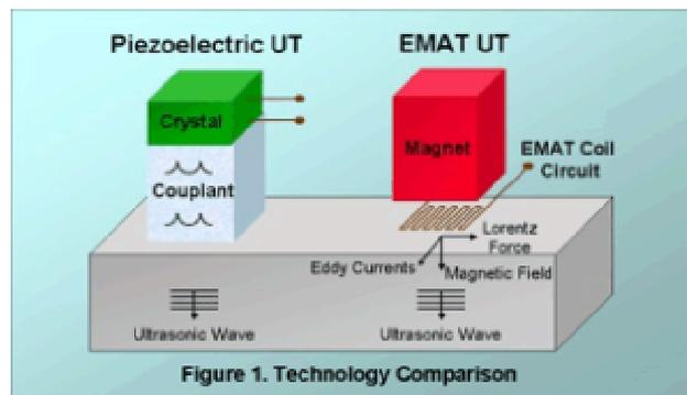
Figure 2. EMAT is couplant-free ultrasonic inspection technique.
