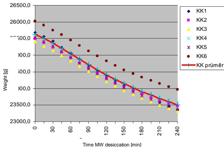
Diagram. 5. The weight decline course of the hollow ceramic brick pieces KERATHERM within MW desiccation. The diagram shows the average weight decline of the brick pieces KERATHERM within MW desiccation.
