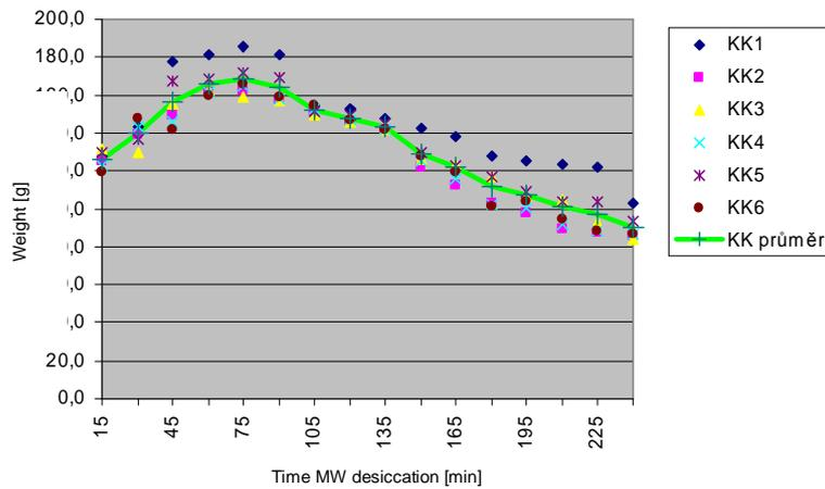
Diagram. 6. The moisture weight loss course of the hollow ceramic brick pieces KERATHERM within MW desiccation. The diagram shows the average moisture weight loss of the brick pieces within the desiccation.
