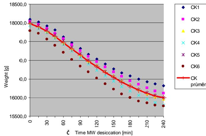
*Diagram. 1. Weight decrements of the separate pillars in the time of MW drying and the curve of the mean decrease of weight of pillars during the MW drying-out made of FBB on LCM*
