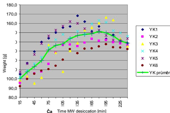
Diadram 4. The process of the weight decrements in YTONG blocks during the MW drying—out and the curve of the mean weight decrements in these blocks during the drying
