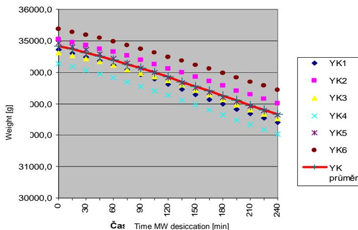
Diagram. 3. Graphic trend of weight decrements of YTONG blocks during the MW drying-out with the marked mean weight decrement
