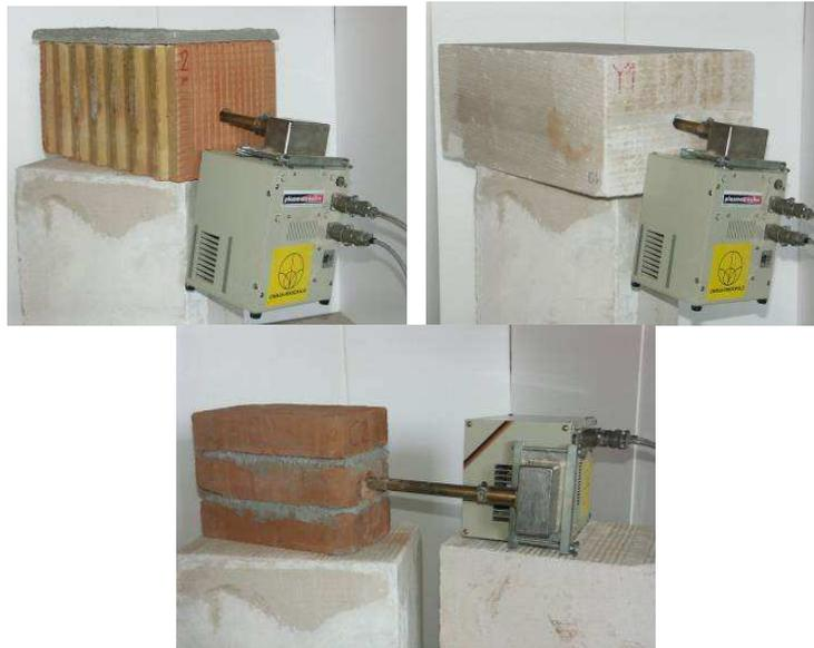
*Fig. 2. Microwave desiccation by means of microwave rod plug-in antenna*
