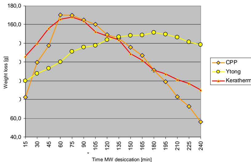
Diagram. 7. Graphic review of the moisture weight loss in particular types of the masonry within MW desiccation.
