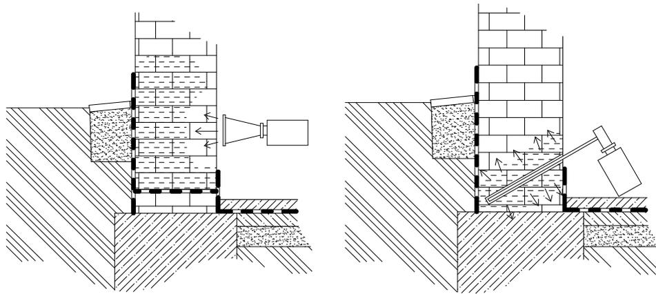
*Fig.1. Microwave desiccation by means of surface funnel antenna and rod plug-in antenna [3]*
