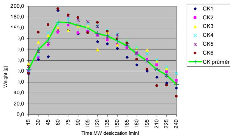
Diagram. 2. The process of decrements of moisture in the pillars of FBB during the MW drying and the curve of the mean decrease of moisture-weight in pillars during the MW drying-out made of FBB
