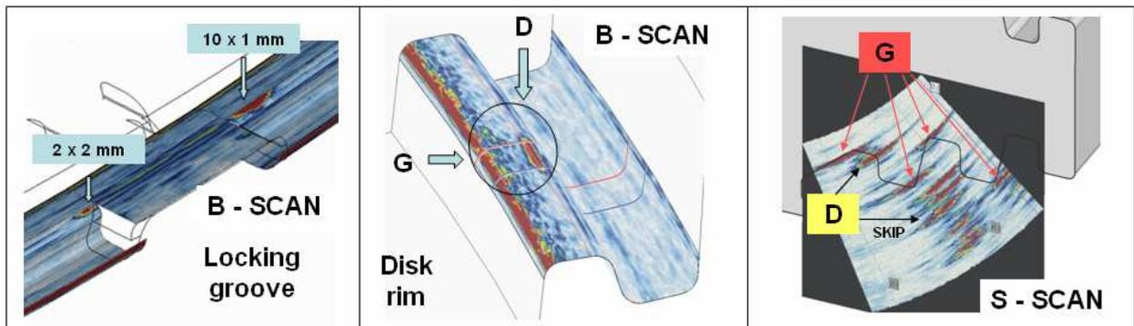
**Figure 1: Examples of bent B-scan (left and middle) and S-scan data plotting for GE disk rim inspection.**
