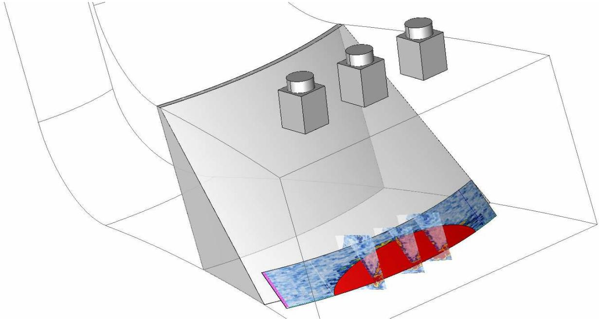
**Figure 5: Example of data plotting, probe position, and defect reconstruction for a crack located in HAZ of a nozzle.**
