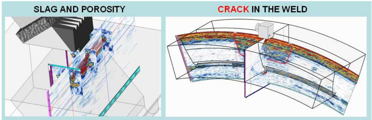
**Figure 7: Examples of data plotting for slag and porosity (left) and weld crack (right) using superimposing B- and S-scans.**
