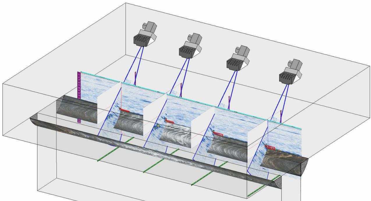
**Figure 8: Data plotting and probe-defect-part relationship for steam generator lug welds. Implanted defect: four toe cracks of different height-same length.**
