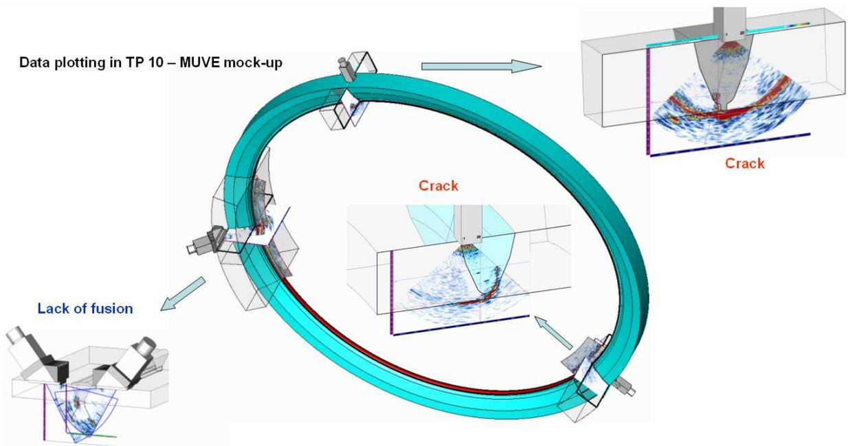
**Figure 6: Example of data plotting for a piping weld mock-up with three implanted defects.**
