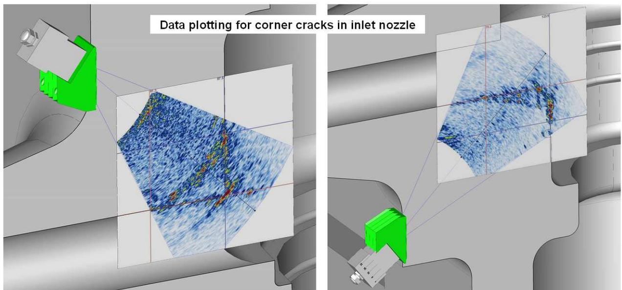
**Figure 15: Example of data plotting for emergency stop valve; crack size and shape for priority 1 (left) and 2 (right) between inlet nozzle and upper chamber.**
