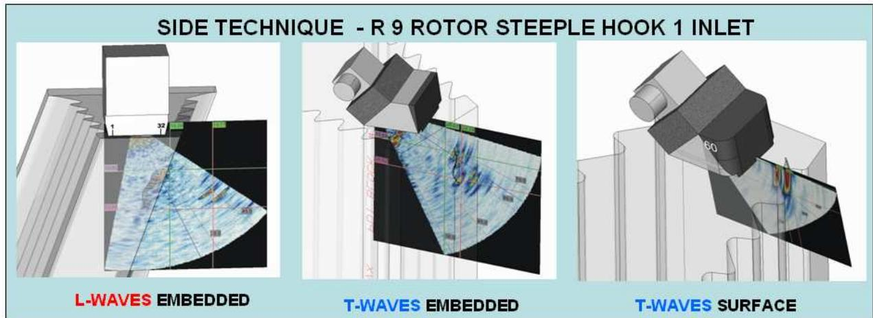
Figure 3: Example of data plotting for side technique applied to Siemens-Parson R9 rotor steeples.
