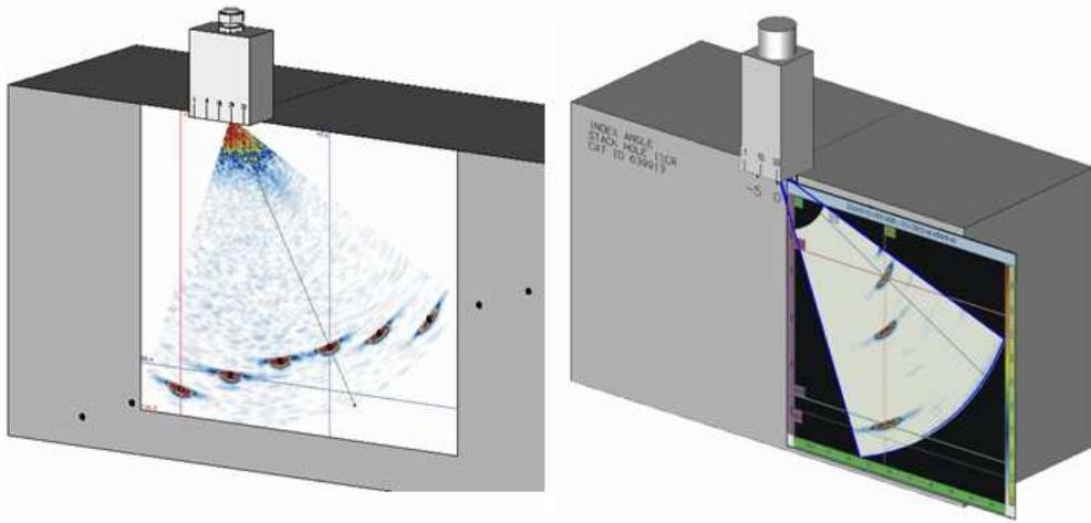
**Figure 12: Examples of data plotting for probe characterization : deeper range [ 60-110- mm ] (left) and shallow depth [ 10-40 mm ] (right)**
