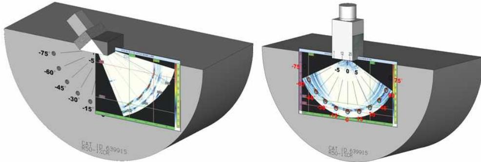
**Figure 11: Example of data plotting for probe characterization - MIC attack set-up - on even-distributed side-drilled holes. Left: T-waves; right: L-waves.**
