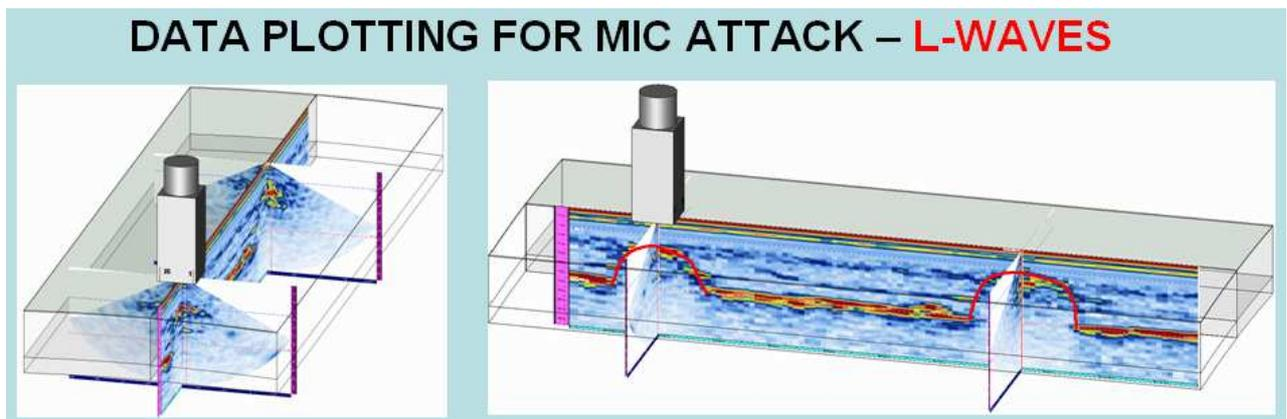
**Figure 13: Examples of data plotting for MIC attack– L-waves on shut down cooler heat exchanger - HAZ of divider plate weld.**
