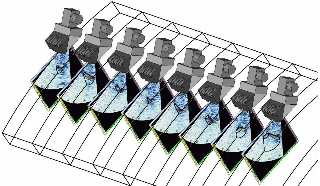
**Figure 14: Data plotting for T-waves on NS-4-10 block with artificial localized MIC defects.**
