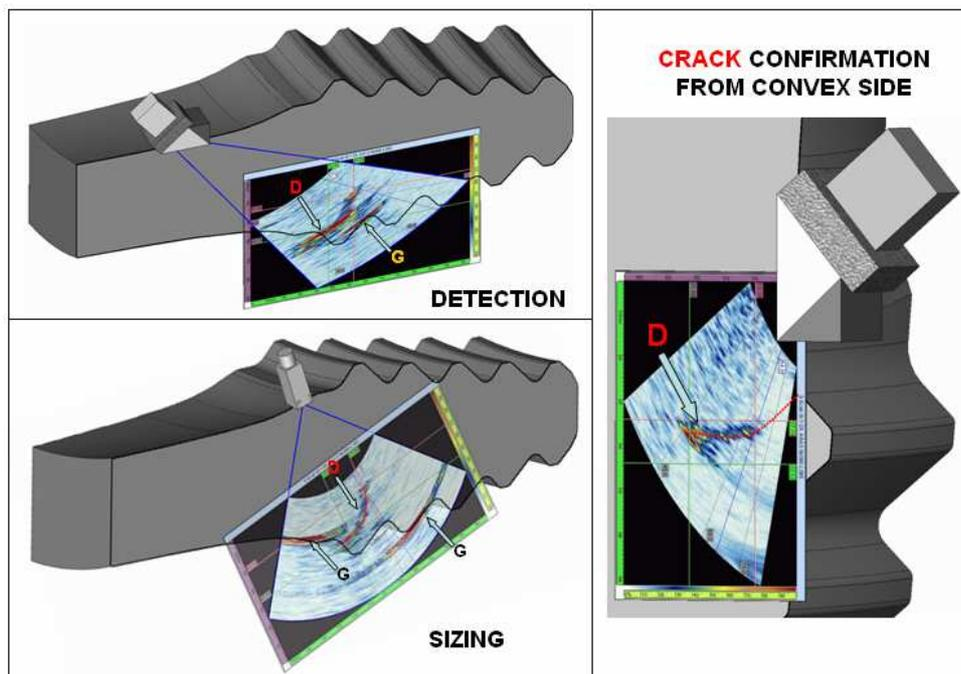
**Figure 2: Example PAUT inspection features (probe, part, defect and S-scan) for crack detection and sizing in L-0 blade (GEC Alstom).**
