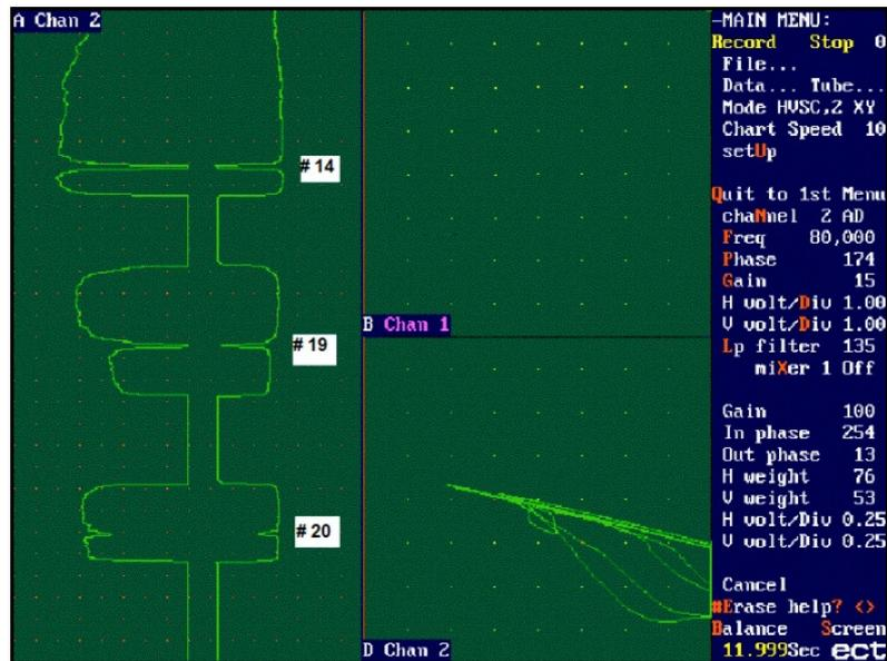
**Figure 4. Different amplitude signals obtained for calibration standards numbers 14, 19 and 20.**
