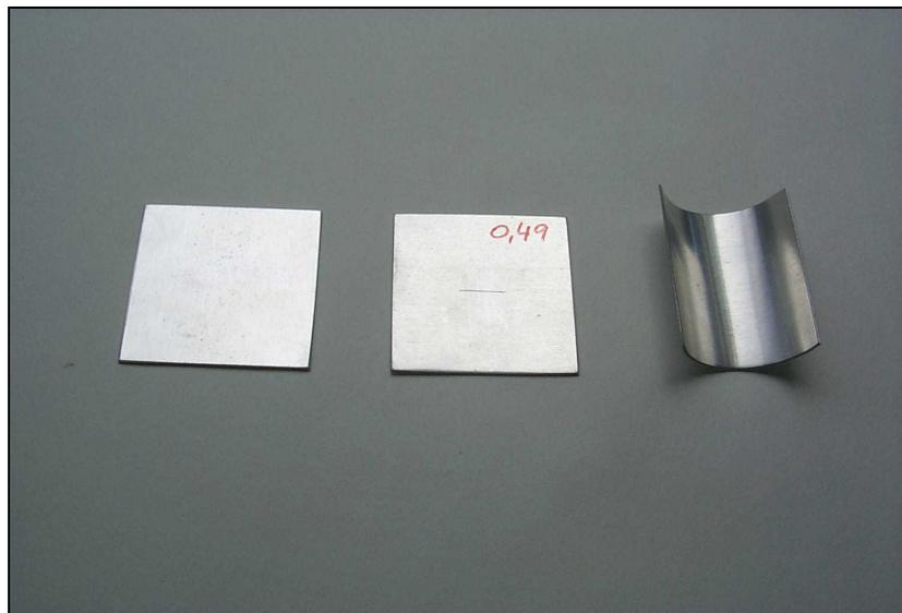
**Figure1. Fabrication sequence for a standard.**
