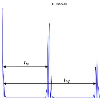
**Figure 4.** Schematic representation of the UT display showing the first two indications.
