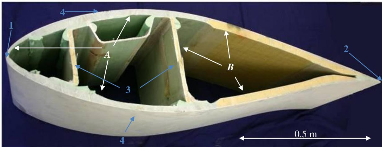
Figure 2: Cross section of a wind turbine blade. The upper side in the picture is called intake side the lower side is called pressure face. On the left the leading edge (1) and the trailing edge (2) can be seen. The bars (3) stabilize the turbine blade and are glued to the belts (4). Large areas are built of GFRP (A). To reduce weight some regions (B) are built as composite of GFRP and wood or plastic foam.
