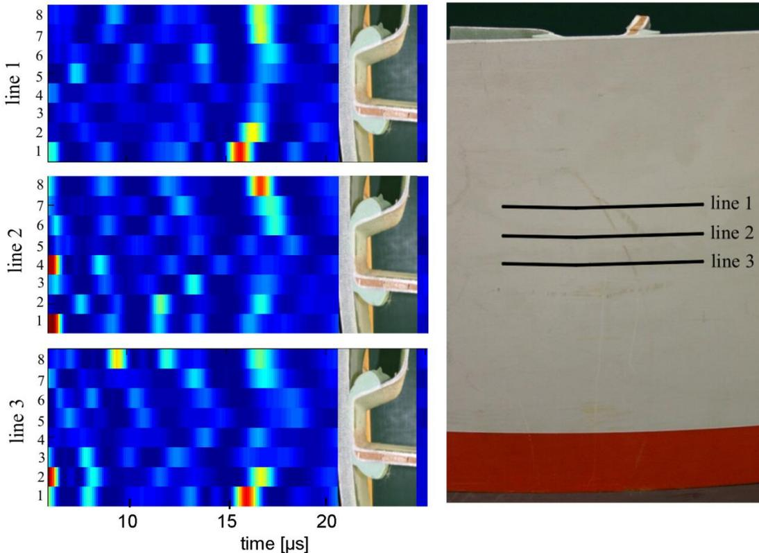
Figure 7: left: energy of the back wall echoes for three measured lines across the bond between bar and belt. Right: Picture of the test specimen and the three lines.
