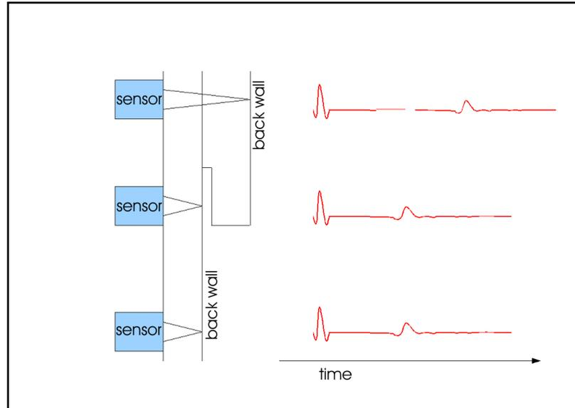
Figure 6: Principle of an ultrasound-echo measurement
