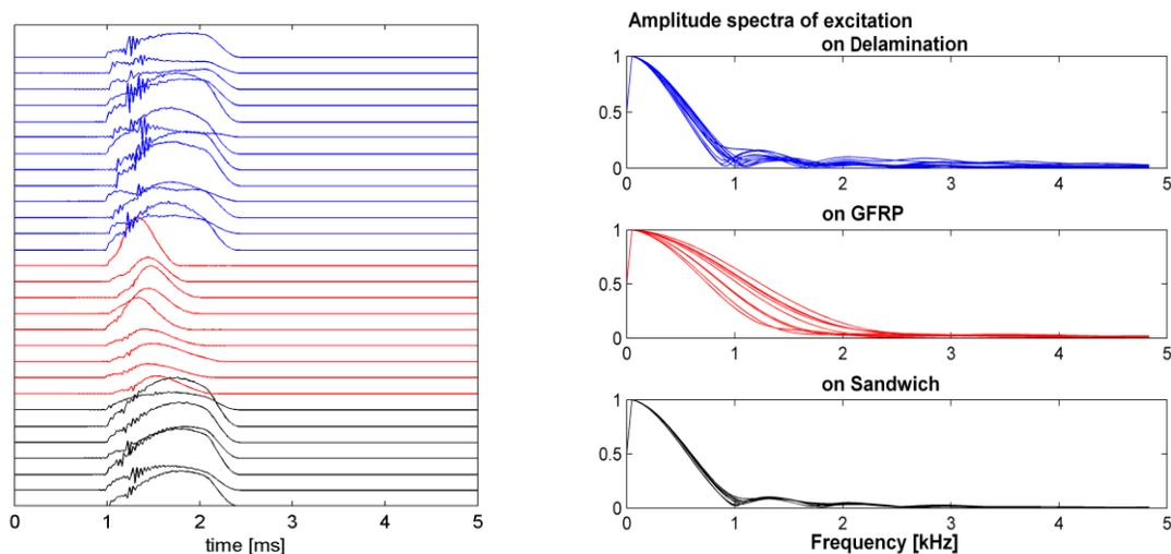
Figure 4: Time data (left) and amplitude spectra (right) of the force recorded at the impulse hammer during an impact. The blue curves (top) show measurements on delaminated GFRP, the red curves (middle) show measurements on intact GFRP and the black curves (bottom) show measurement excited on Sandwich areas.
