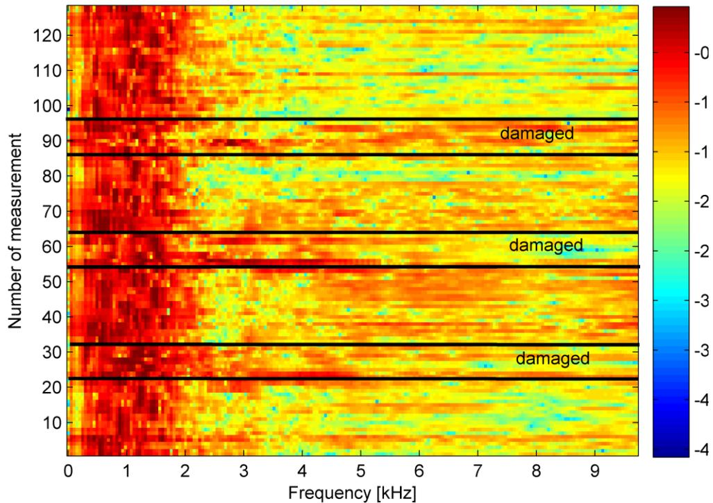
Figure 5: Logarithmic amplitude spectra of the recorded sound at 128 impact points.
