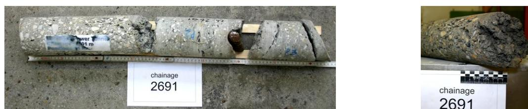
Figure 8: Concrete core from chainage 2691
