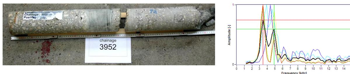
Figure 9: Concrete core from chainage 3952 (left is inside) and corresponding FFT from the centre point
