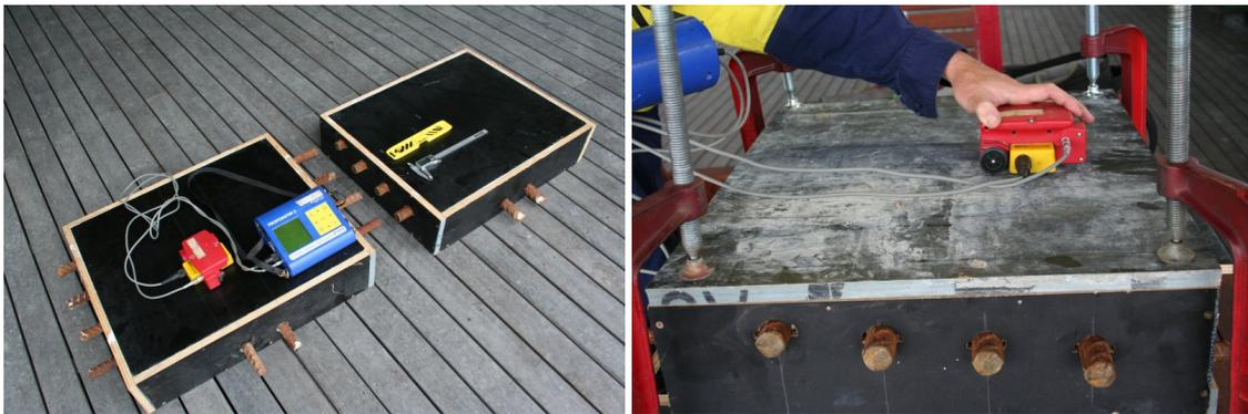
Figure 2 a) Calibration blocks with N24 & N28 bars, b) Scanning of bars using Profometer 5 Scanlog
