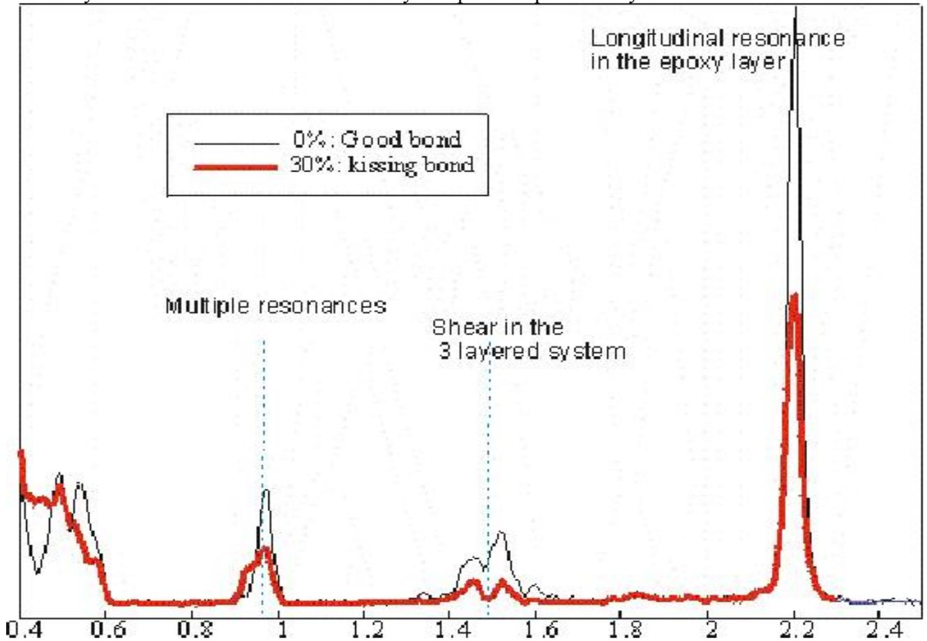
Figure 4: Spectra from the Quasar RI 2000 for a good bond (black line, 0% contamination) and for a kissing bond (30% contamination, red line).
