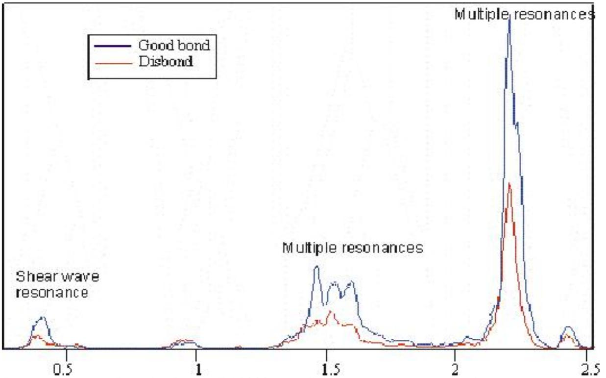
Figure 5: Spectra from the Quasar RI 2000 recorded on two positions over the titanium diffusion bond sample showed on figure 3. The blue line represents the spectrum over a well-bonded area of the diffusion bond (good bond, blue line) and the red line (disbond) shows the spectrum recorded over the region where the alpha case layer is located.
