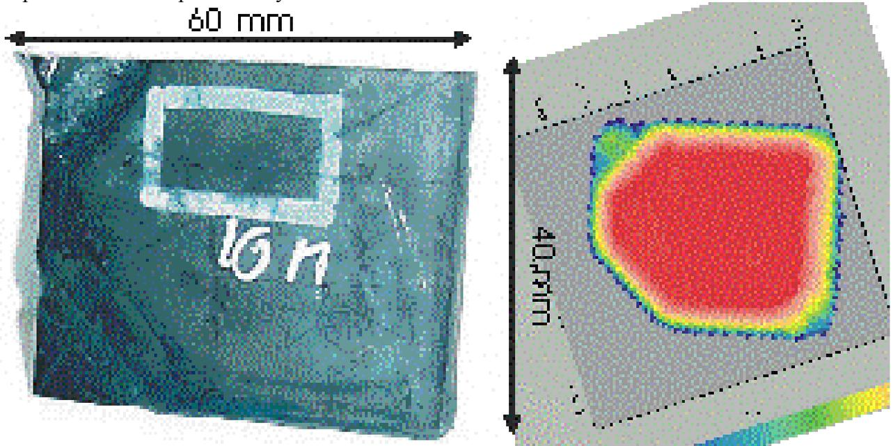
Figure 1: Titanium diffusion bond with indication of the position of the alpha case layer, and the C-scan at 10MHz.
