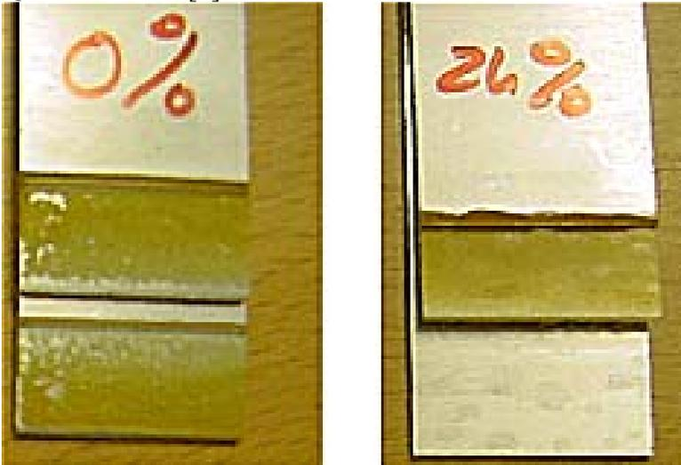
Figure 3: failure mode for the good bond (0% contamination) and the kissing bond (24% contamination).
