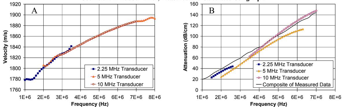
A measurable increase in compression wave velocity was observed with increasing frequency, going from 1800 m/s at 2 MHz to almost 1900 m/s at 8 MHz. As seen for other viscoelastic materials, the velocity does tend to level off at high frequencies where relaxation effects play a diminishing role.
