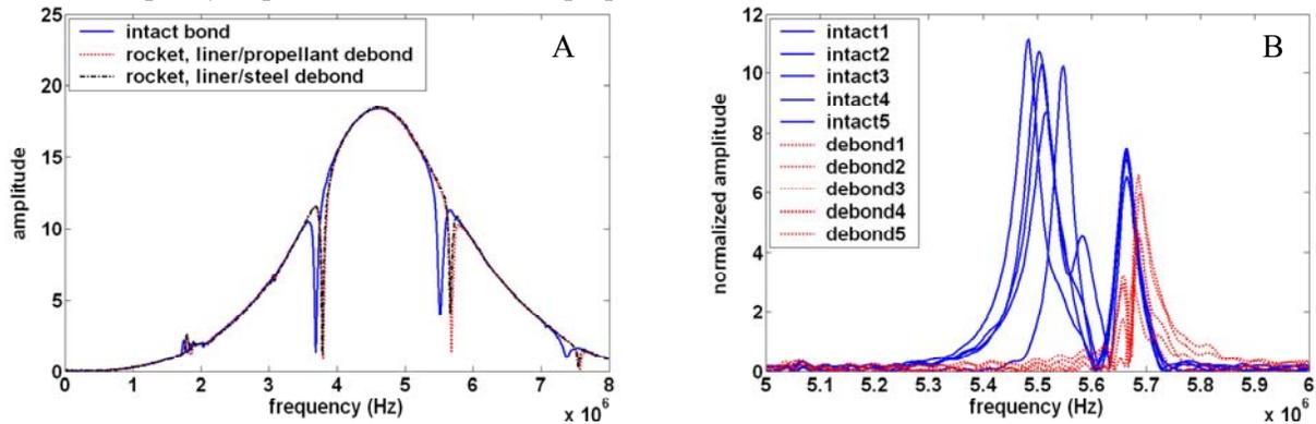
The same normal beam compression wave tests were performed on the rocket specimen, which produced similar results as presented in Figure 7. The shift in resonant frequency is more pronounced than seen previously for the flat samples. The larger shift in resonant frequency resulted in the double peak in the difference spectrum of Figure 7-B.
