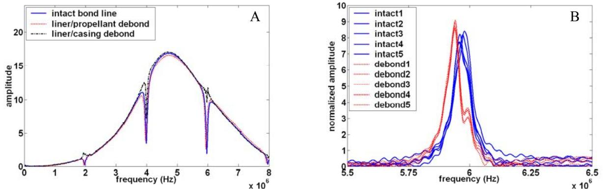
Alternatively, one could de-convolve the responses of an intact bond and debond at the fuel-rubber interface using that of the steel case (debond at the steel-rubber interface) as a reference. This would be equivalent to taking a transfer function approach. One should be able to detect the contributions of the liner and propellant to the total signal, provided that the signal-to-noise ratio is adequate in the frequency domain responses. The drawback to this proposed technique is the
