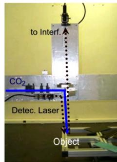
Fig. 2: Coupling device of the INCA platform that guides the laser light on the object
