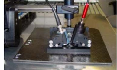
Fig. 10: laser US portable head from Dassault in pitch-and-catch configuration
