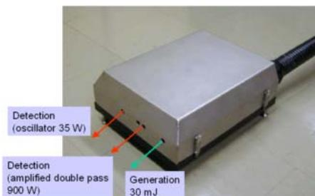
Fig. 6: Laser US head by IMI integrating generation and detection laser in a 30x30cm<sup>2</sup> device
