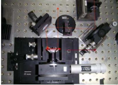
Fig. 4: Onera optical parametric oscillator for 3.1-3.4 $\mu$ m laser light generation
