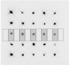
Fig. 8: Multi-channel by LCF/IO laser US. Picture of the image of the 25 detection points with detector line scheme
