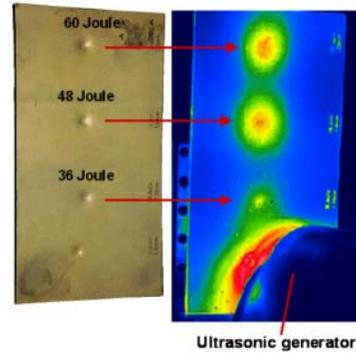
Fig. 14: Use of ultrasonic excited lock-in thermography for impact detection on a GFRP/metallic laminate (9 metal layers) with debondings
