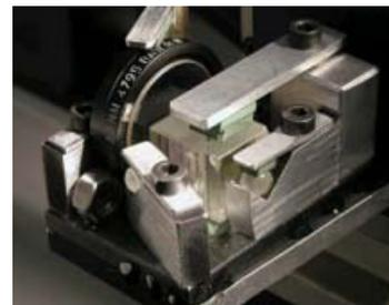
Fig. 7: CESI coupling device of the fibre post-amplifier
