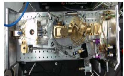
Fig. 3: View into the opened thin disk laser demonstrator for laser US applications
