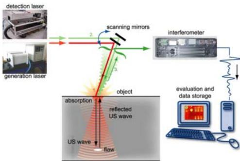
Fig. 1: Laser-coupled ultrasonic testing principle. In INCA the guiding mirror are replaced by a XY-translation stage
