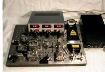
Fig. 5: CESI optical parametric oscillator for mid-IR laser light
