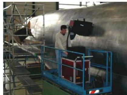
Fig. 12: INCA Shearography demonstrator in in-service use on a real aircraft
