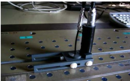
Fig. 11: First version of a GMR sensor used for cracks detection on lap joints of metallic laminates
