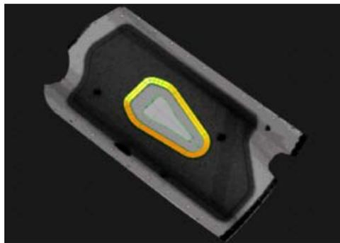
Fig. 15: X-ray picture mapped on a digital, CAD based object representation
