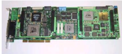
Fig. 9: Laser US data acquisition and evaluation board
