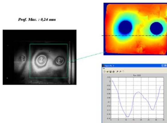
*Fig. 8 : Result : rivet pull-in on aircraft fuselage*
