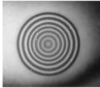
*Fig. 3 : the shadow moiré applied to the analysis of dents*
