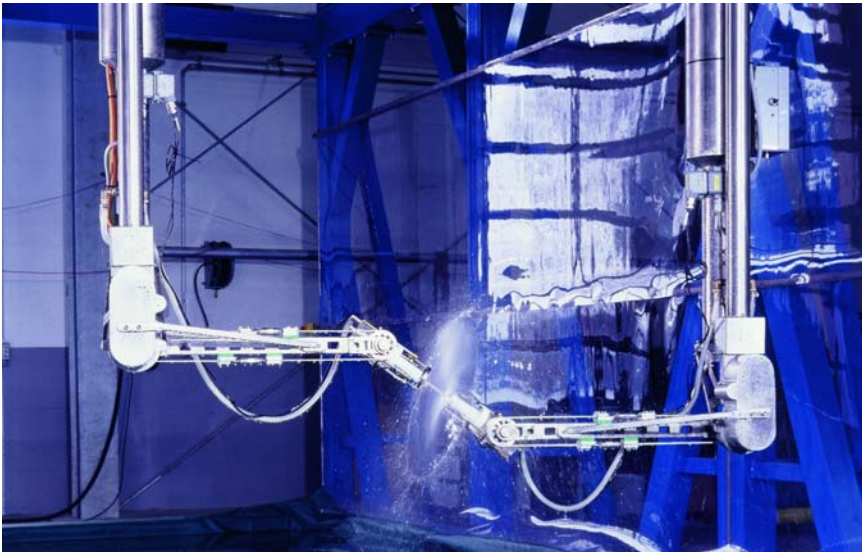
(Slide 5: Special capability: Test of cranked parts with extender arms)
