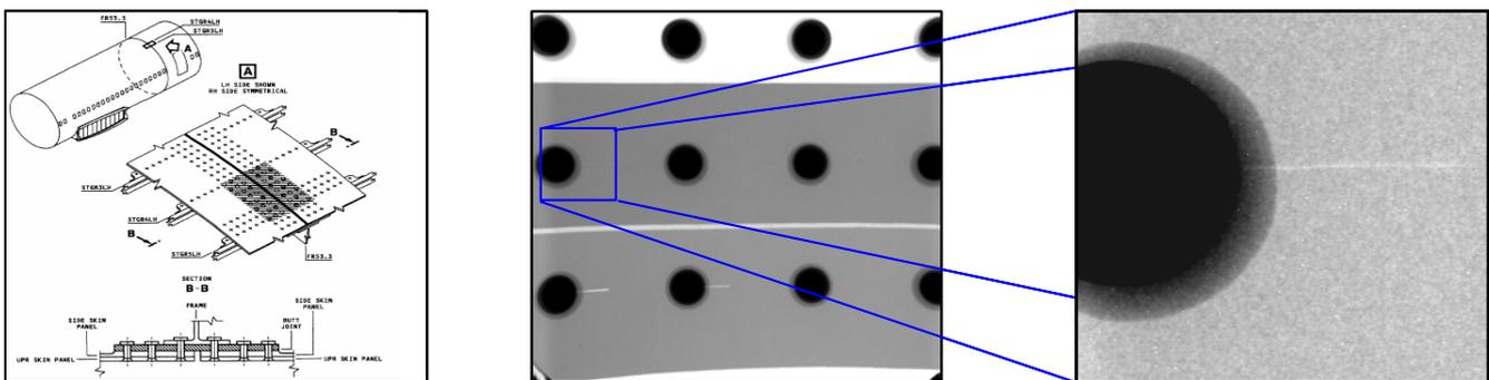
Figure 3 - Lap joint with electro-eroded and fatigue cracks: zoomed image - fatigue crack of 0.1mm opening.
