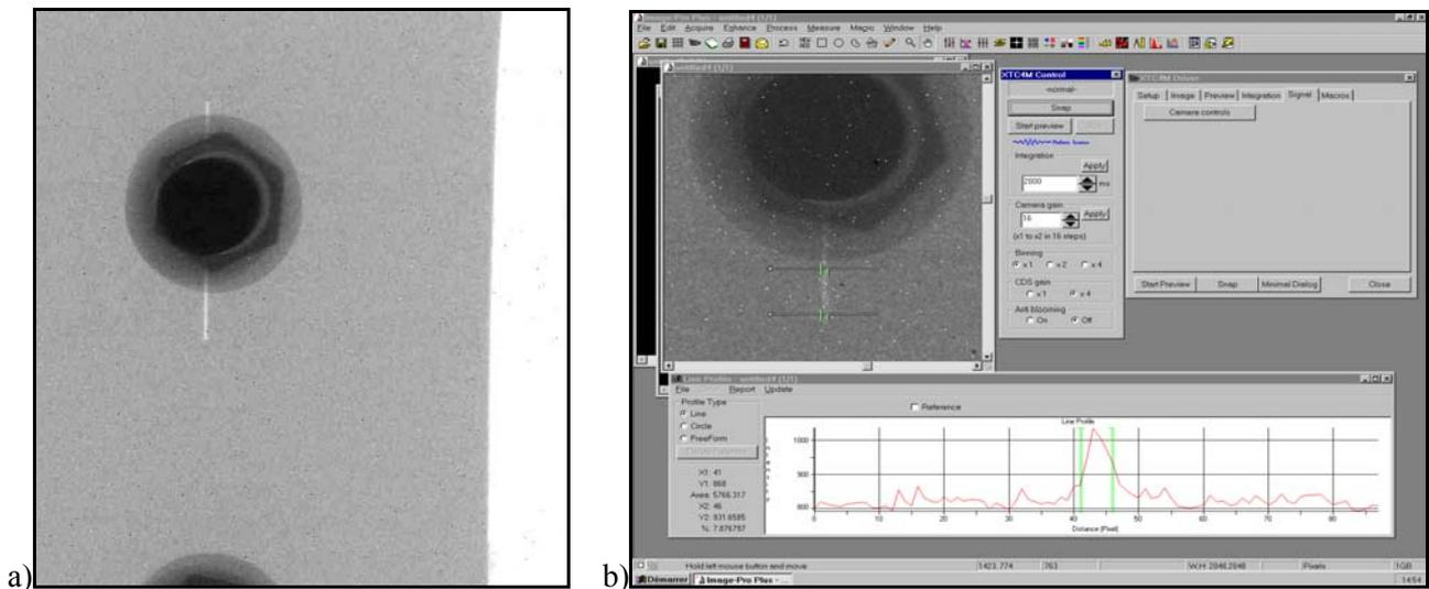
Figure 6 – a) X-ray image of crack under rivet. B) User interface with measuring tool.
