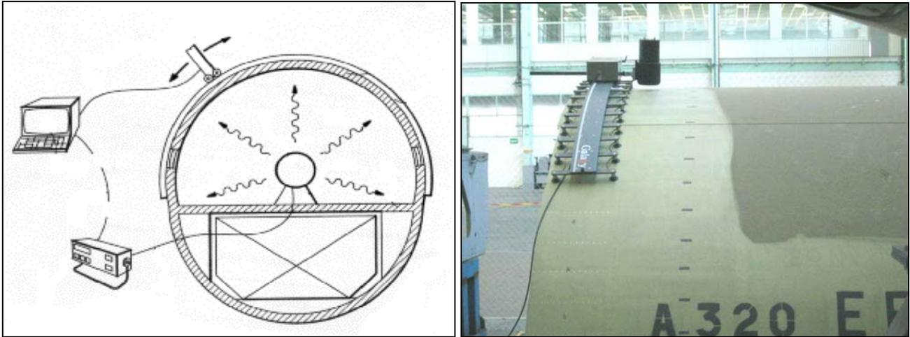
Figure 4 – Foreseen application for the XHINIA system: in service circumferential assembly inspection.
