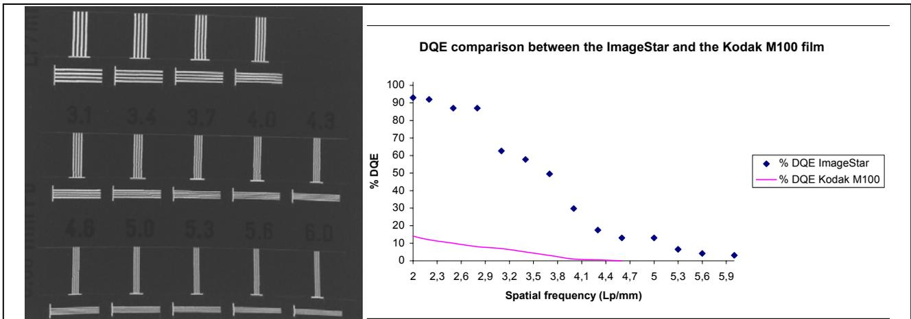
Figure 2 – Line pair phantom image for detector characterization and comparison of DQE detector performances (ImageStar VS Kodak M100 film @ 80 kV).
