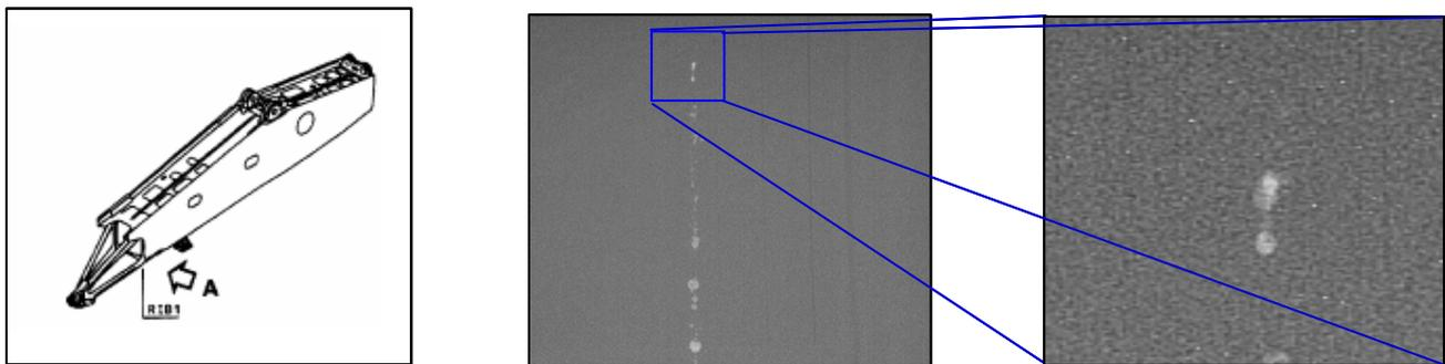
Figure 7 – Engine spar 25mm titanium weld with flaws: zoomed image – gas holes of 0.8mm diameter.
