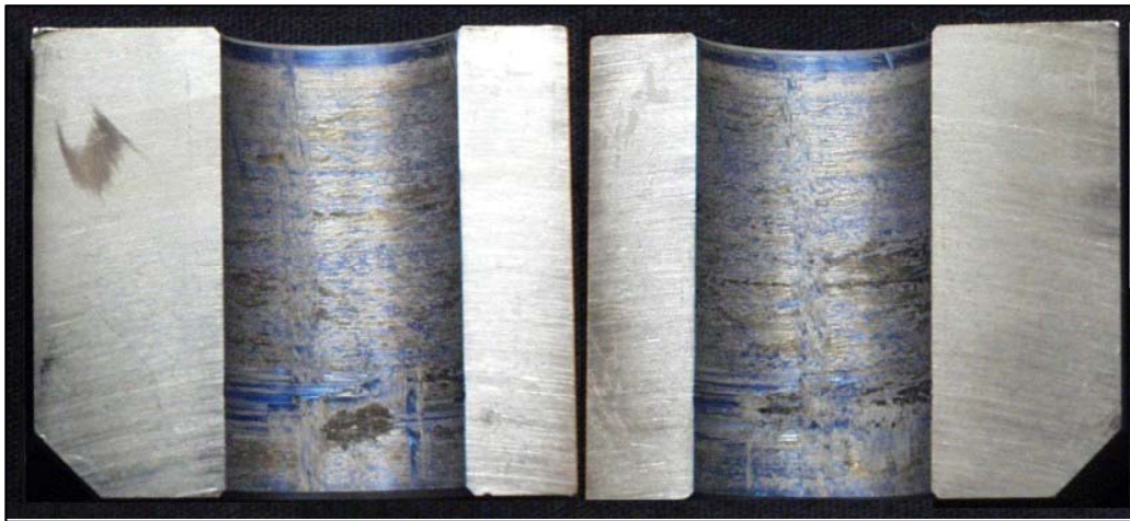
Figure 4. Photograph of inner surface of sectioned titanium sample
