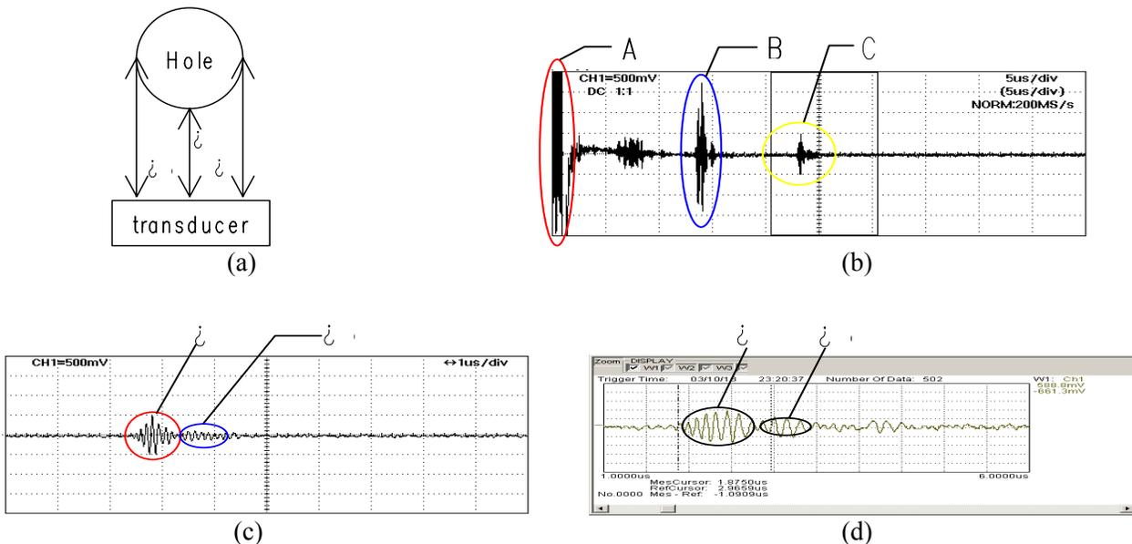
Fig. 4 A result of hole sizing: (a) the schematic of different paths of reflected SAW's, (b) reflected SAW signals recorded at oscilloscope, (c) a zoomed detail of the part C, and (d) a further zoomed detail of part C.
