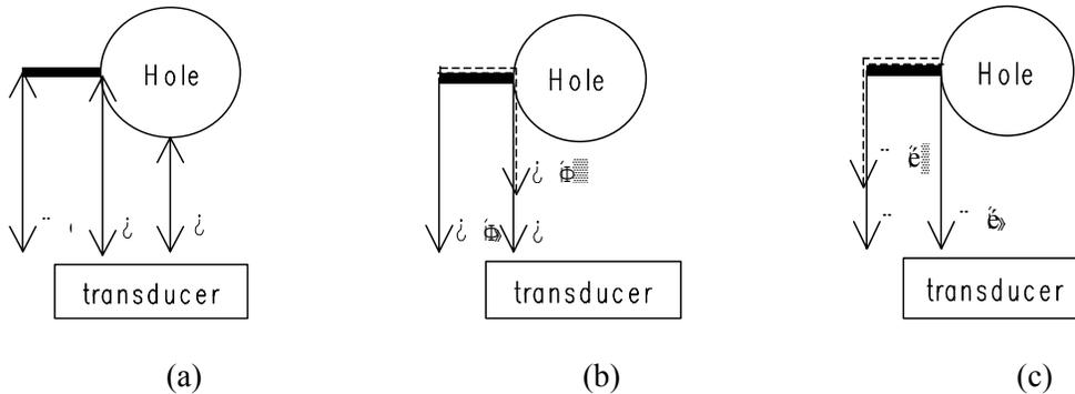
Fig. 6 Schematics of the path of reflected SAW's: (a) three different paths of plausible reflections of SAW's, (b) various paths of SAW-2, and (c) various paths of SAW-3.
