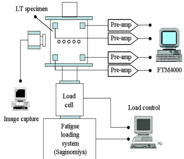
Fig. 2 A schematic diagram of experimental set-up
