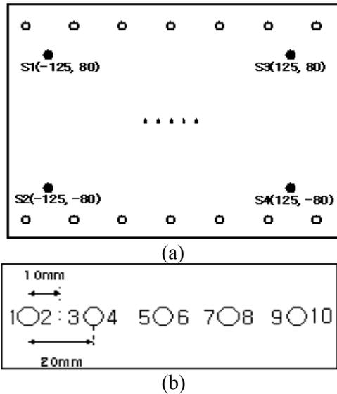
Fig. 1 Geometry of specimens; (a) rivet holes with an array of AE sensors and (b) numbering of prospective crack sites
