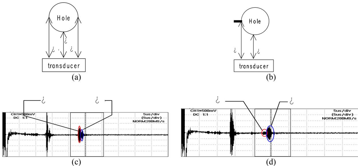
Fig. 5 A result of crack detection: (a) the schematic path and (c) the signals of reflected SAW's with no crack, and (b) the schematic path and (c) the signals of reflected SAW's with a crack.
