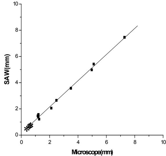
Fig. 8 Comparison of the crack length determined by the SAW technique with the measured values by travelling microscope.
