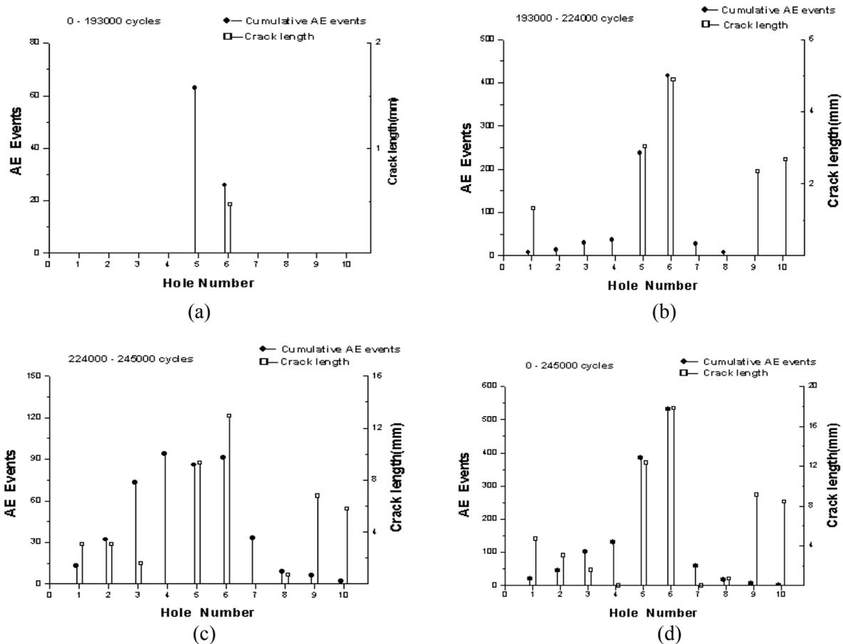
Fig. 3 The incremental crack growth and cumulative AE events at individual site; (a) during 0~193000 cycles, (b) during 193000 ~224000 cycles, (c) during 224000~245000 cycles, and (d) during the entire fatigue test
