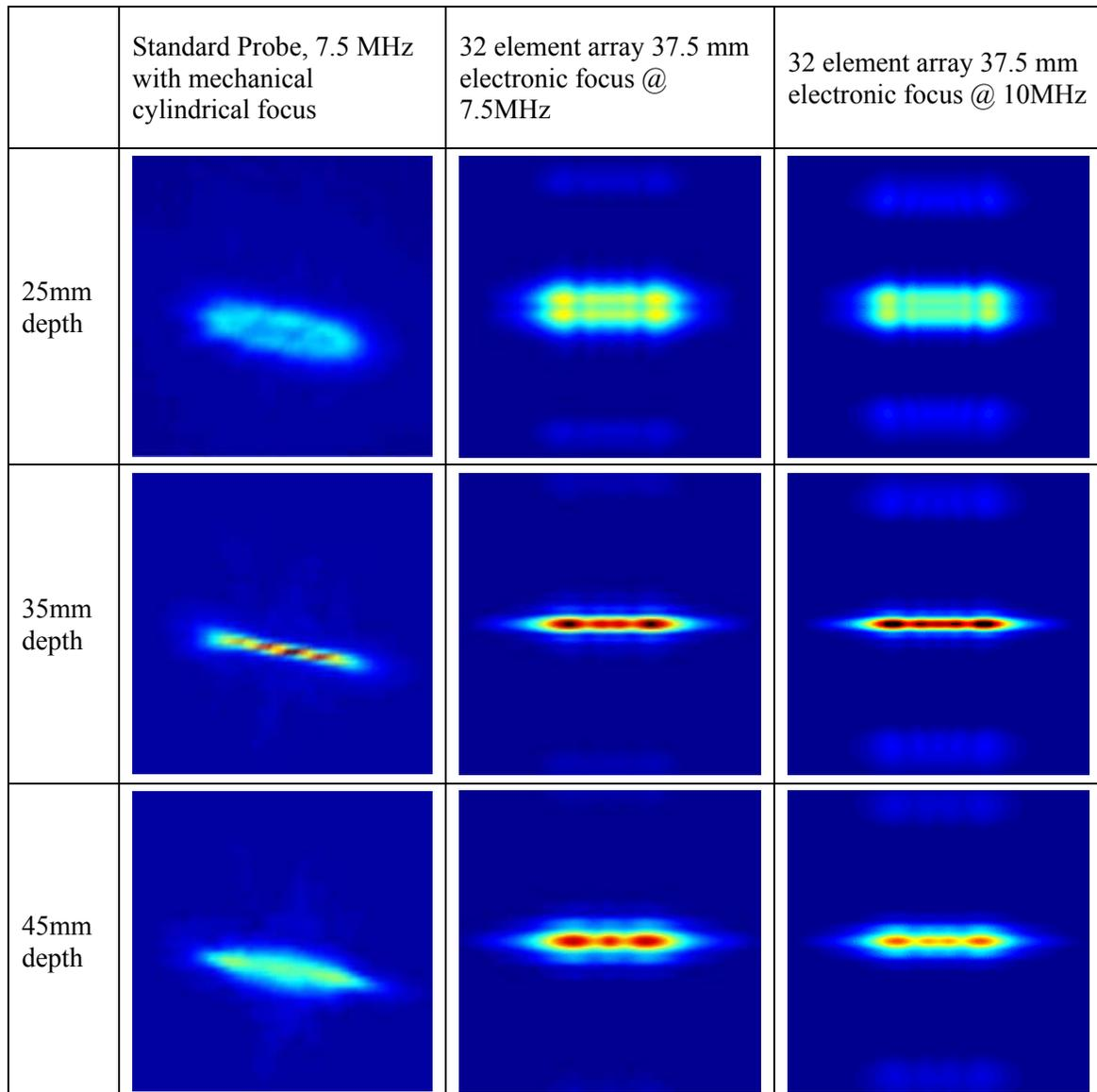
**Figure 4:** Comparison between measured sound field for a conventional probe and simulated sound field for two possible array configurations.
