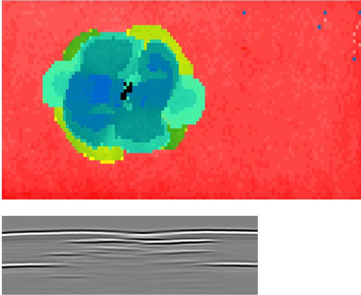
**Figure 9:** C-scan thickness image of impact damage for a 5 mm thick carbon fibre skin showing cross section B-scan view through central region of impact.
