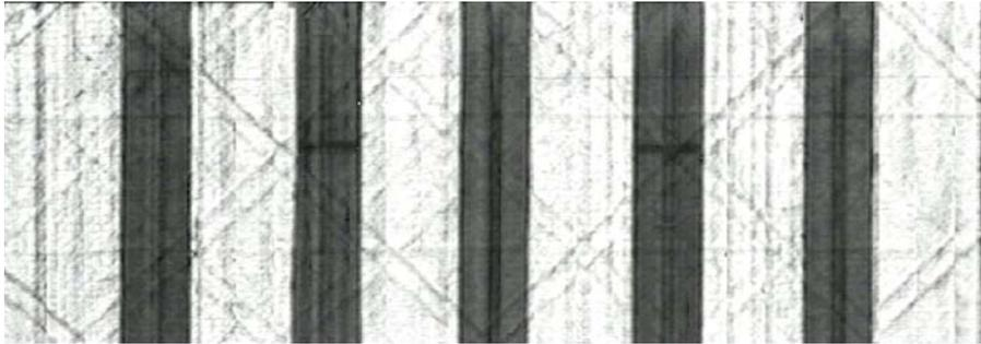
**Figure 11:** Large area RapidScan image of composite wing skin and bonded stringers.
