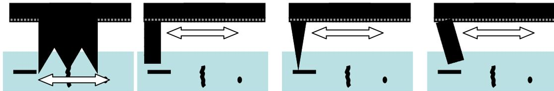
Figure 1: Phased array scan modes with sector scan and raster scans.
