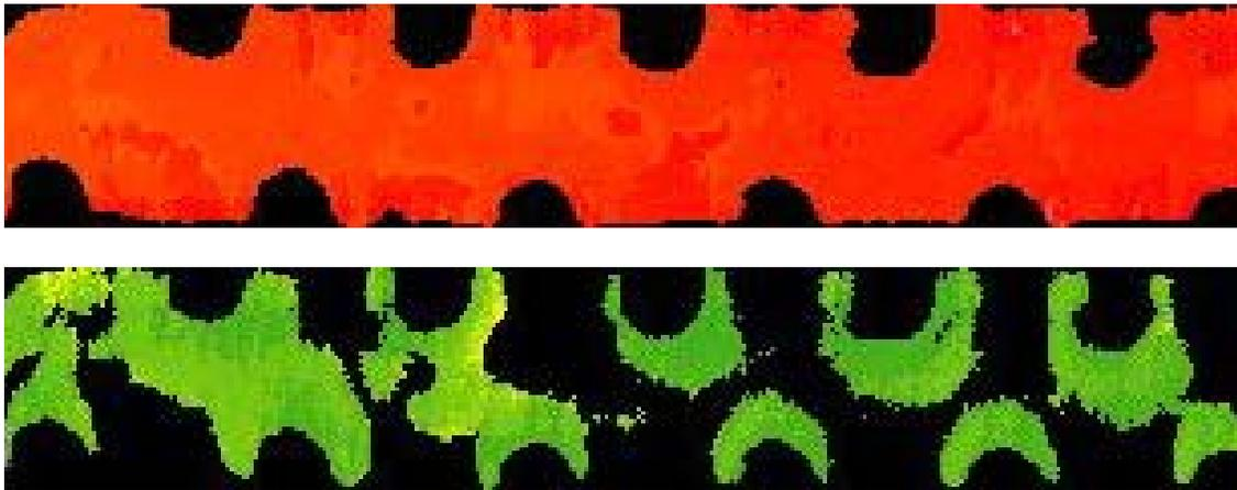
**Figure 7:** Scan of sealant bonding showing coupling check scan (top) and sealant bonding check (bottom)
