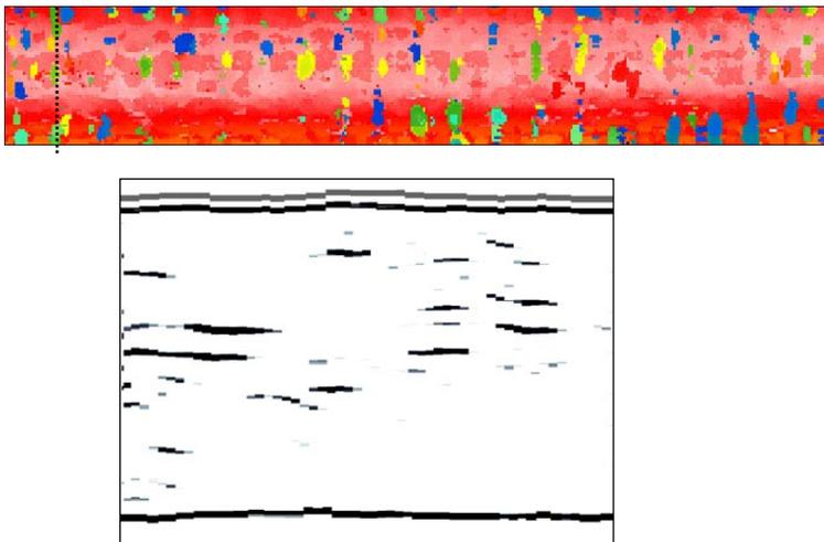
**Figure 10:** C-scan image of porosity in 5 mm cured pre-preg and cross section B-scan of porosity showing depth and extent of porosity.
