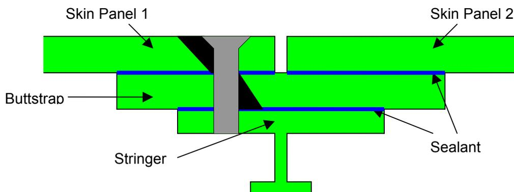
**Figure 6:** Typical wing skin joint configuration showing sealant and fastener locations. Possible crack locations are shown in black to the left and right of the fastener.
