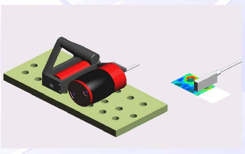
**Figure 2:** Rapid C-scan generation with an array housed in a water filled wheel probe.
